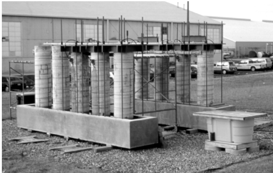
Figure 2.9 Column Corrosion Test Setup 2
