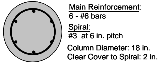
Figure 2.2 Reinforced Concrete Column Section Details 2
