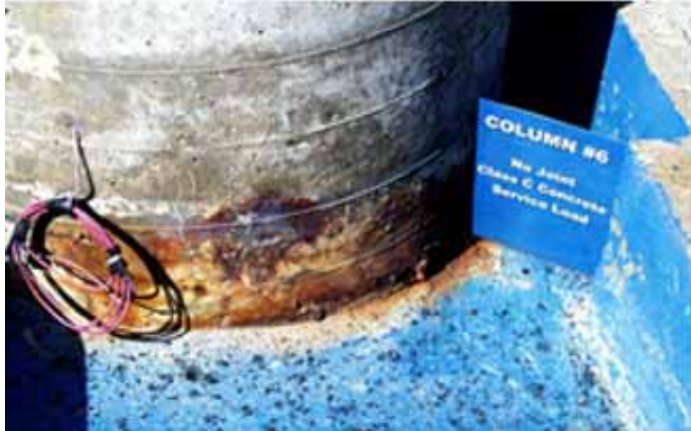
Figure 4.15 Condition of Specimen NJ-TC-S at the End of Testing 1
