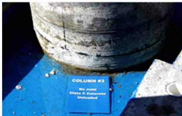
Figure 4.7 Condition of Specimen NJ-TC-N at the End of Testing 1
