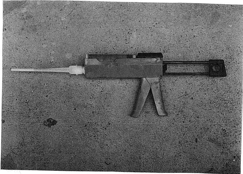
Figure 3.16 Two-component cartridge and nozzle in applicator.
