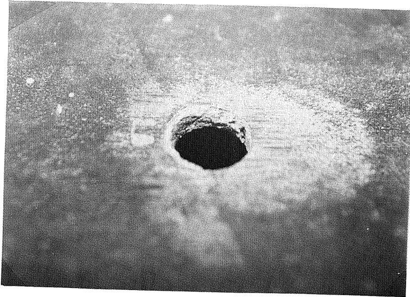
Figure 4.6 Surface abrasion on steel section.
