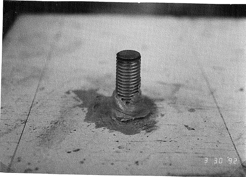
Figure 3.20 Epoxy applied to base of anchor bolt.
