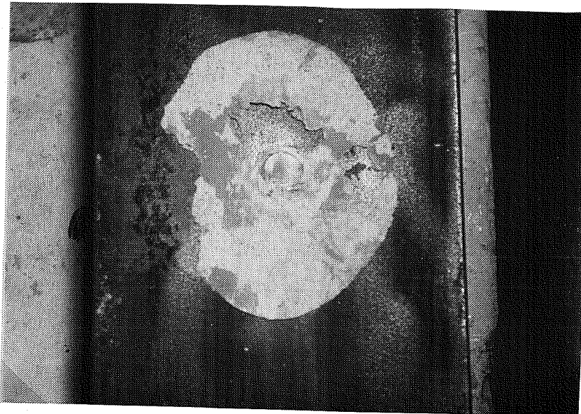
Figure 4.19 Failure of epoxy at both concrete and steel surfaces – Test Me3t.
