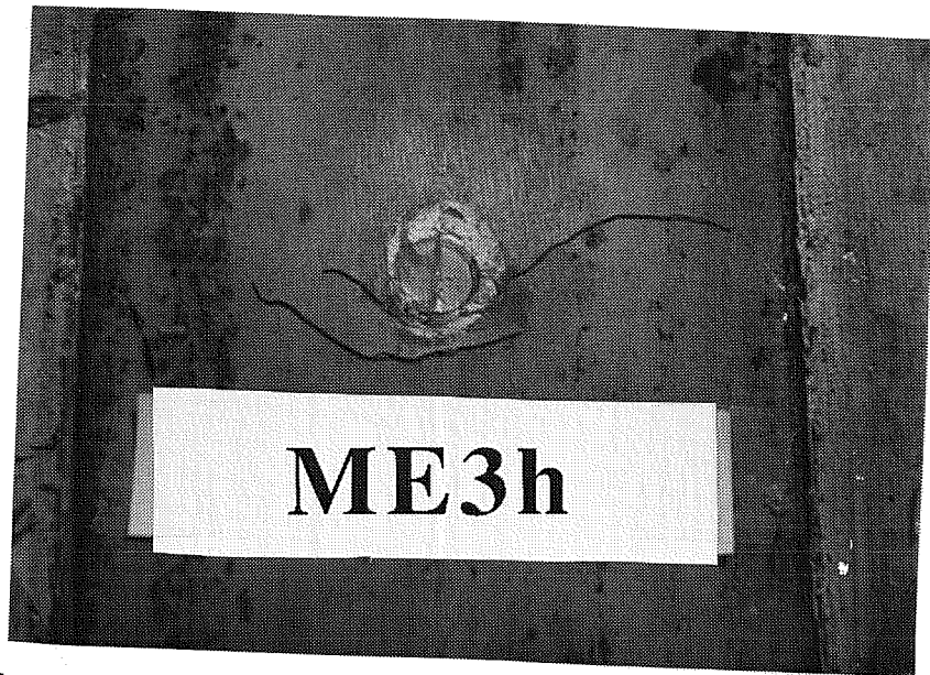
Figure 4.33 Cracking in tension of interface epoxy – Test ME3h-SS.
