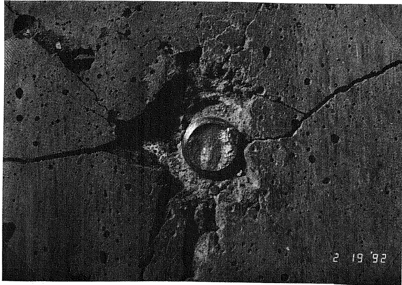
Figure 4.69 Interface cracking and grout crushing – Test CG3T-SS.
