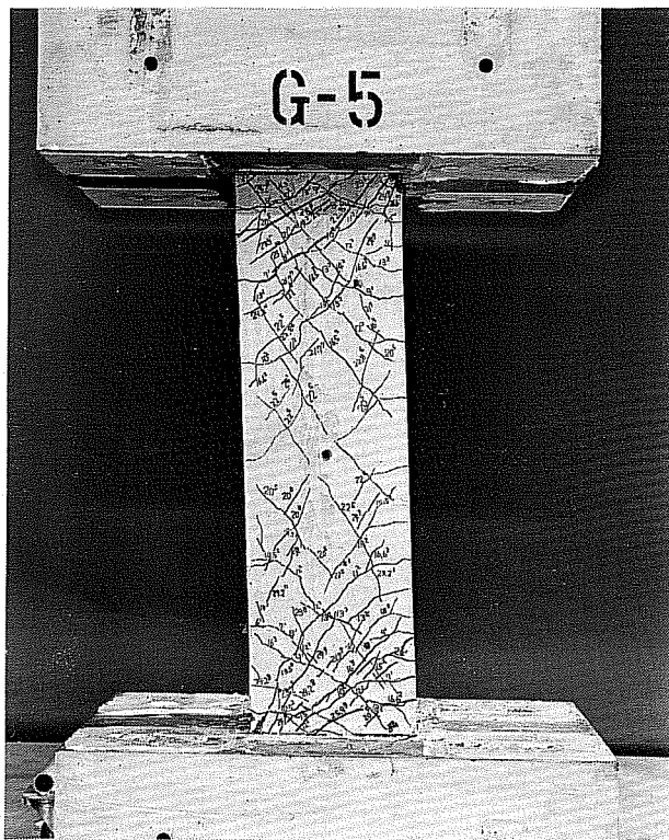
Fig. 13 Final Crack Pattern of Beam Specimen
