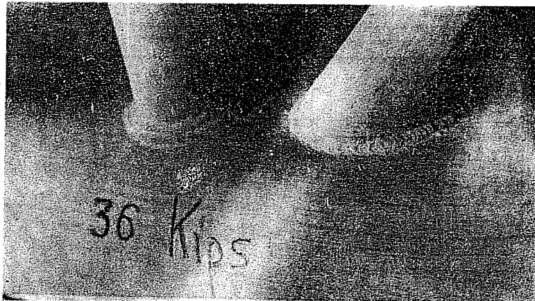
Fig. 4.20 Static load failure in K-joint (series B) with extended braces
