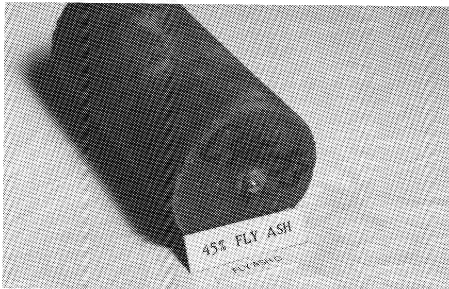
Photo 5.4 Concrete specimen containing 45% fly ash C at 137 days.
