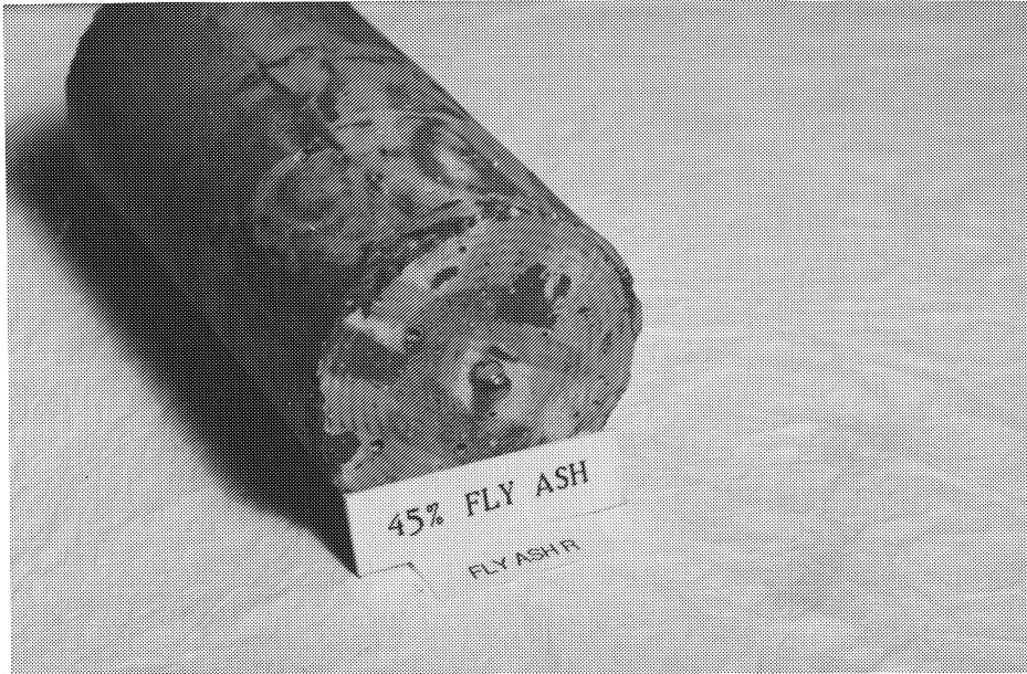
Photo 5.11 Concrete specimen containing 45% fly ash R at 151 days.
