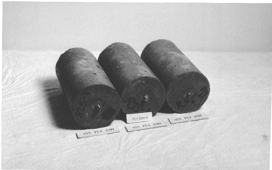
Photo 5.16 Comparison of concrete specimens containing fly ash R with 25, 35 and 45 percent replacement by volume.
