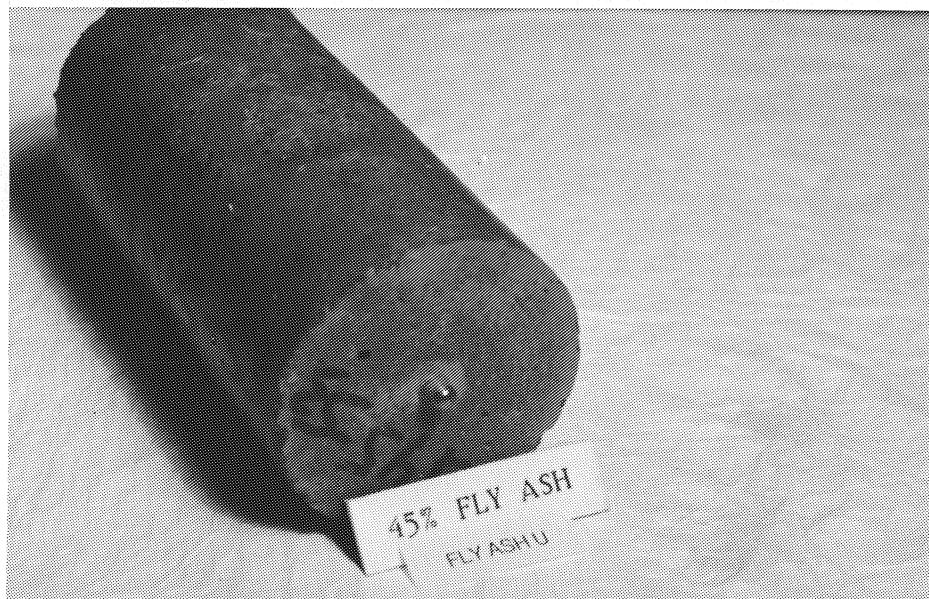
Photo 5.14 Concrete specimen containing 45% fly ash U at 120 days.
