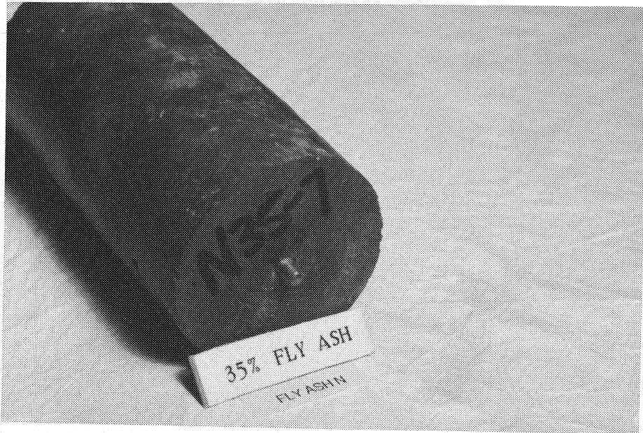
Photo 5.9 Concrete specimen containing 35% fly ash N at 42 days.
