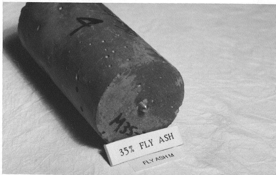
Photo 5.8 Concrete specimen containing 35% fly ash M at 151 days.
