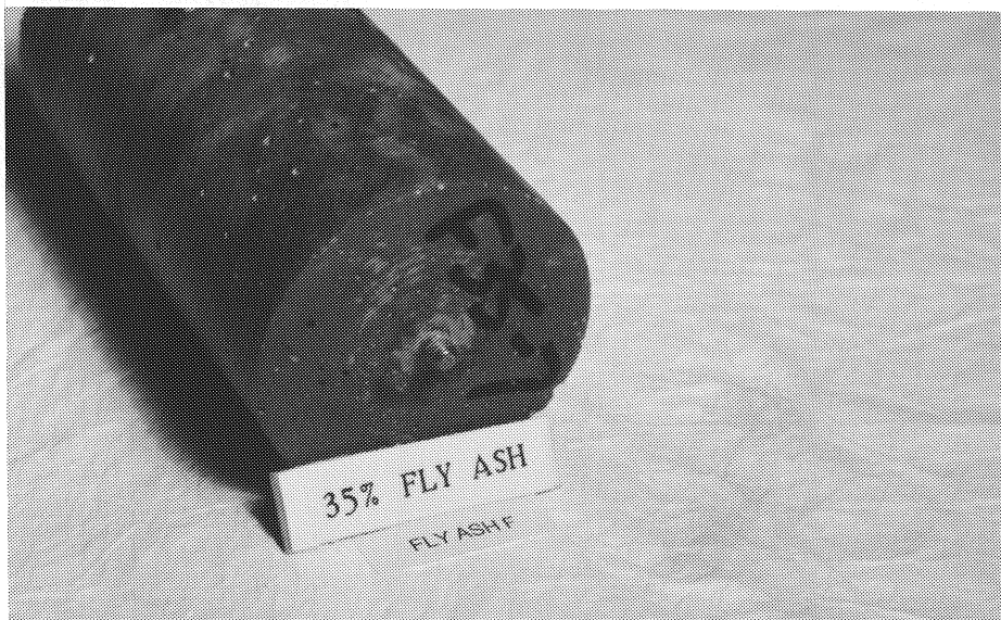
Photo 5.6 Concrete specimen containing 35% fly ash F at 56 days.
