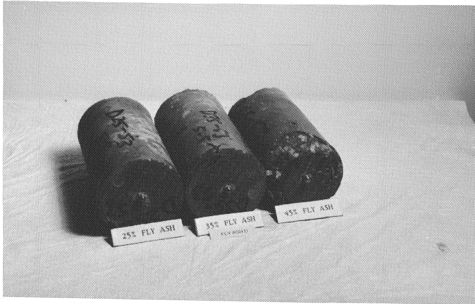
Photo 5.17 Comparison of concrete specimens containing fly ash D with 25, 35 and 45 percent replacement by volume.
