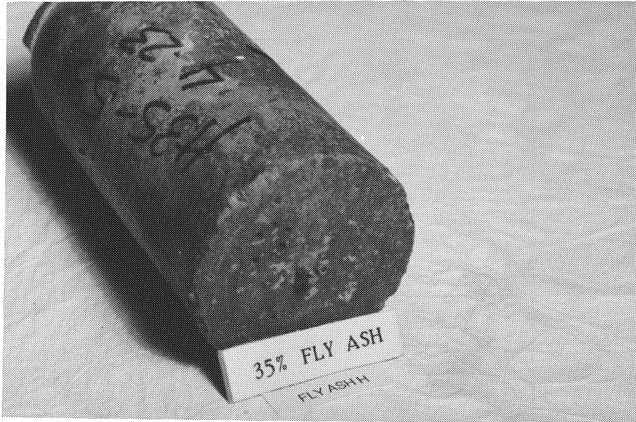
Photo 5.7 Concrete specimen containing 35% fly ash H at 169 days.
