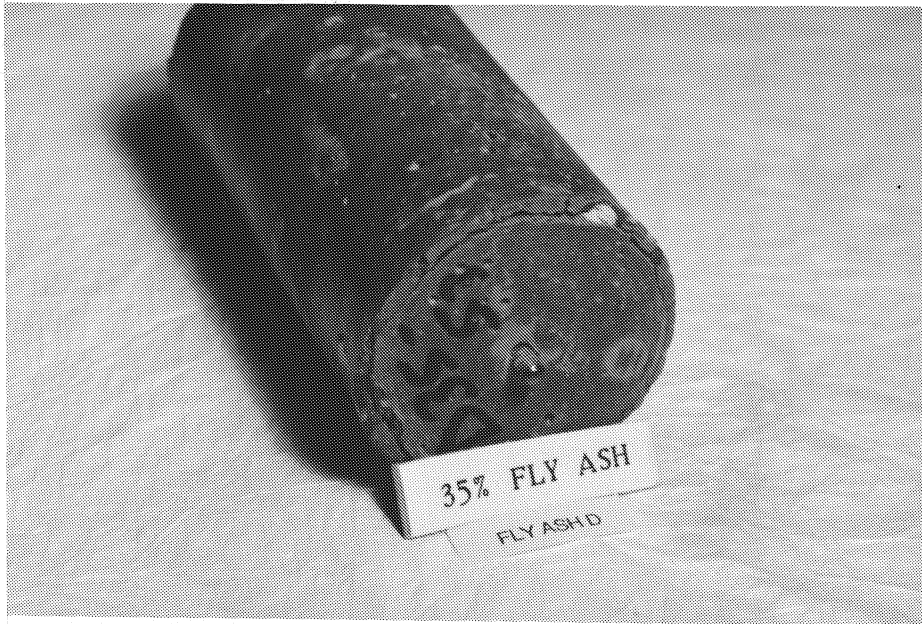
Photo 5.5 Concrete specimen containing 35% fly ash D at 165 days.
