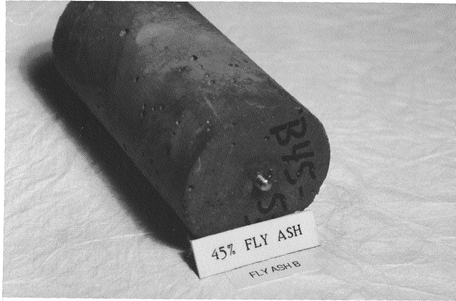
Photo 5.3 Concrete specimen containing 45% fly ash B at 137 days.
