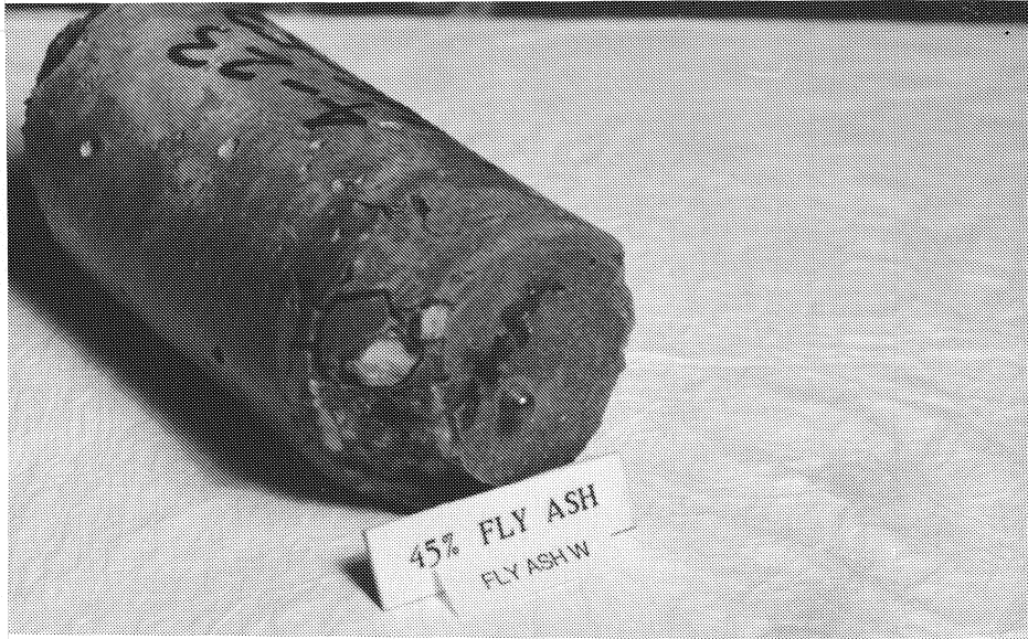
Photo 5.15 Concrete specimen containing 35% fly ash W at 165 days.
