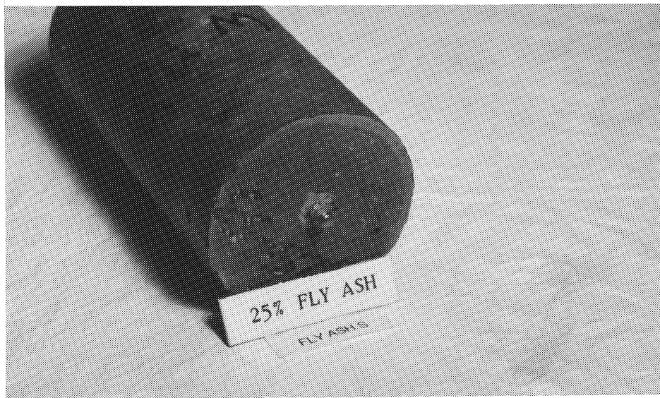
Photo 5.12 Concrete specimen containing 25% fly ash S at 119 days.
