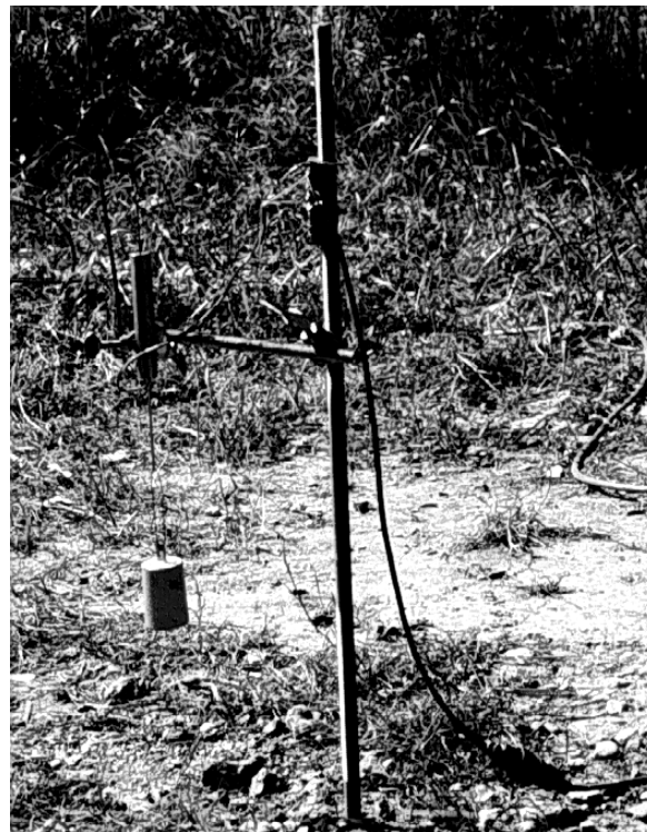
Figure 3.13 DCDT Mounted on Rod
