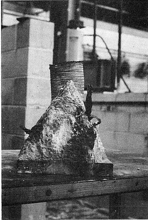
(i) Cone of crushed concrete, still attached to anchor, removed from specimen after failure
