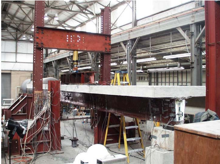
Figure 3.5 - Trapezoidal Hand Lay-up Beam with Concrete Deck
