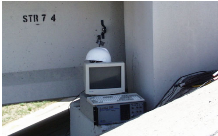
Figure 4.2 – LOCAN 320 Instrument Being Used to Monitor Traffic Noise
