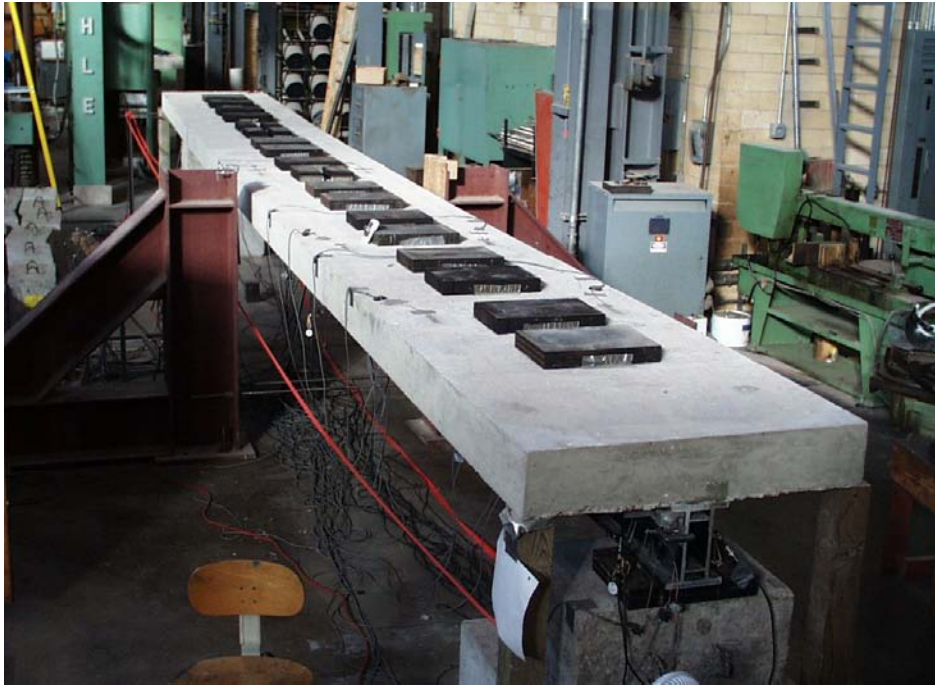
Figure 3.3 - Carbon Fiber and Glass Reinforced Vinyl Ester Pultruded Beam with Concrete Deck
