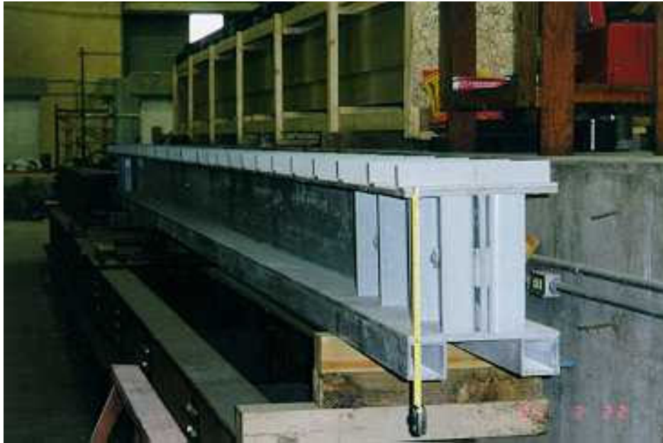
Figure 3.1 - Glass Fiber Reinforced Isophthalic Polyester Pultruded Beam with Shear Connectors, Prior to Casting Reinforced Concrete Slab
