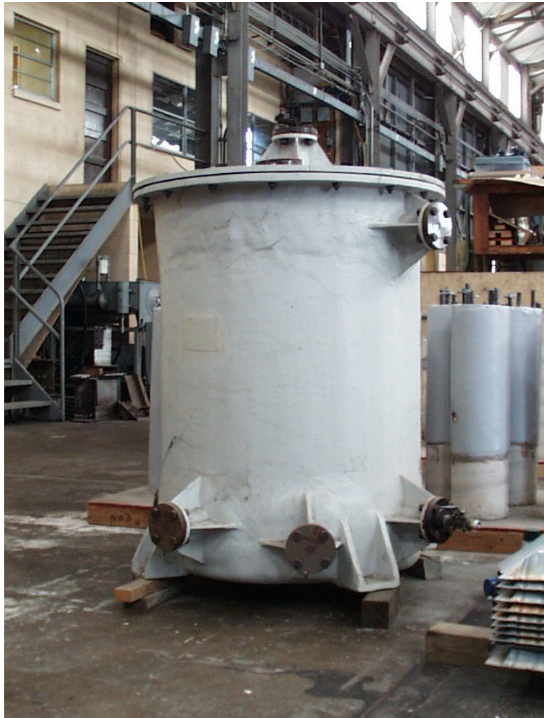
Figure 3.8 – Contact Molded FRP Vessel with In-service Damage
