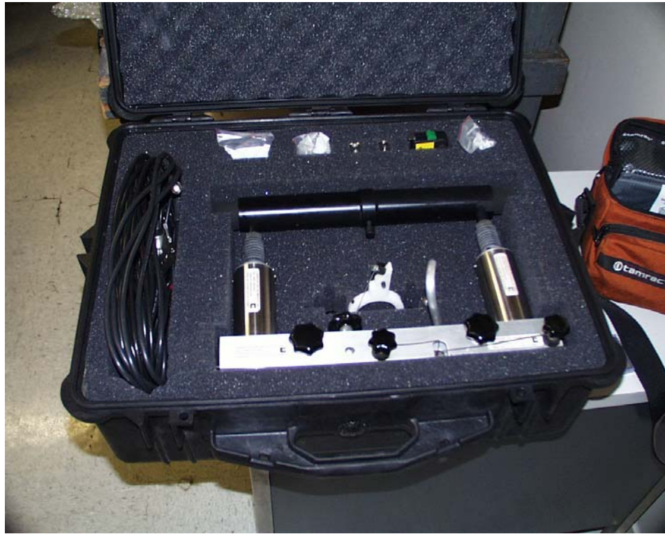
Figure 6.9 – Photo of DOctor Impact-Echo Equipment
