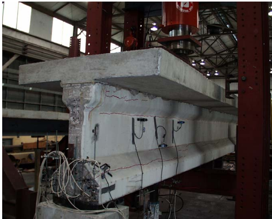
Figure 2.6 – View of Type C Girder with Slab Prior to Testing
