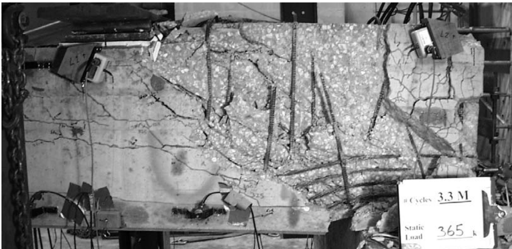
Figure 4.30 Failure of the west web of BG3S after 3,328,600 load cycles and a 365 kip (1620 kN) quasi-static load
