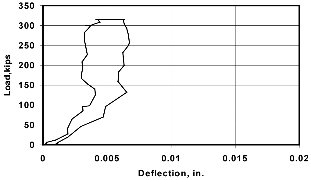
BG3N - North Bearing Pad (East Web)
