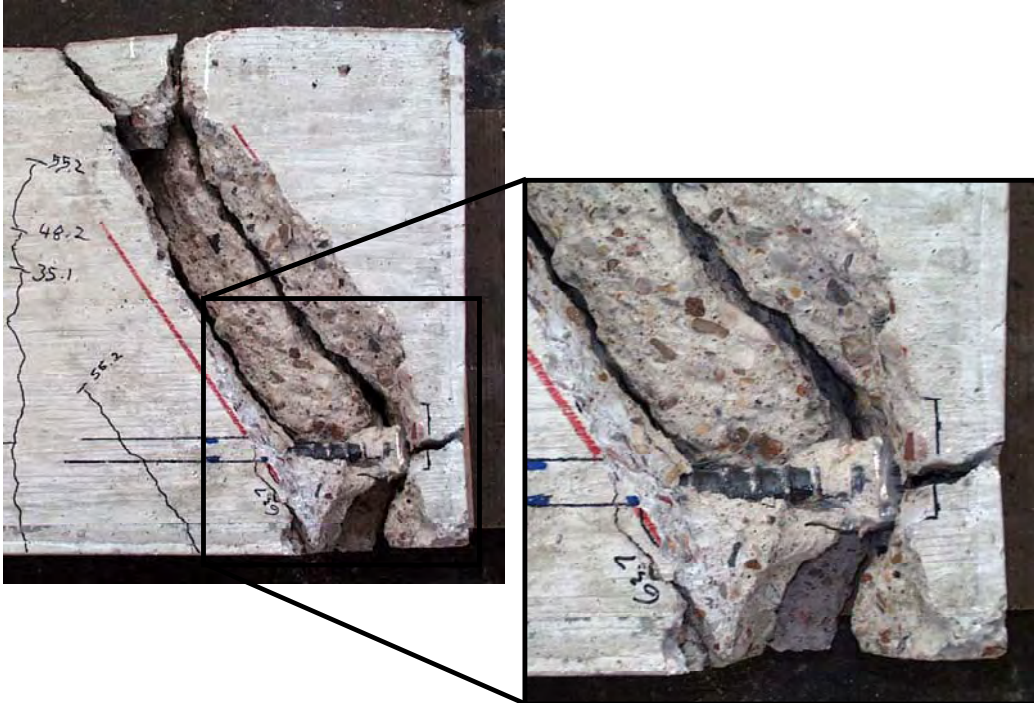
Figure 3-24: Side view of a failed specimen with a vertically oriented head (CCT-08-55-02.80(V)-1) demonstrating splitting of the diagonal compression strut
