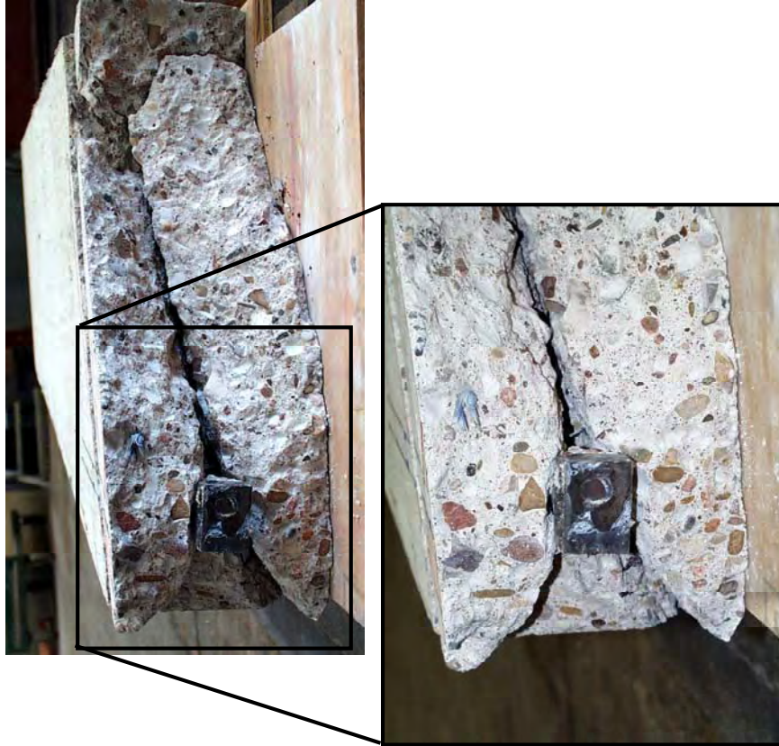
Figure 3-25: Front view of a failed specimen with a vertically oriented head (CCT-08-55-02.80(V)-1) demonstrating splitting of diagonal compression strut
