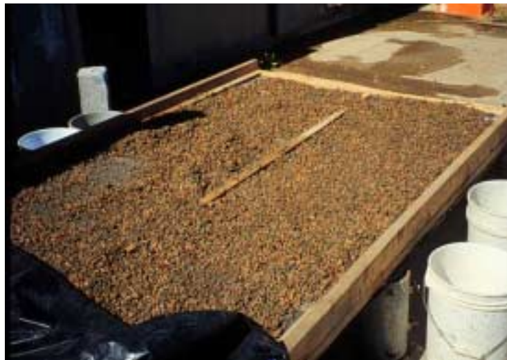
Figure 3.20 Drying of Aggregate on Screened Bed
