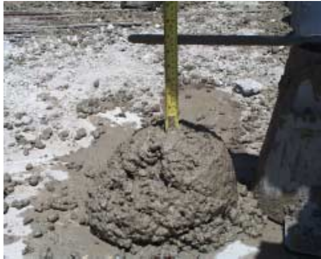
Figure 4.9 Slump of Second Batch of 6000 psi Concrete
