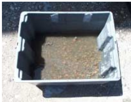
Figure 3.1 Aggregate Soaking in Tub Before Drying
