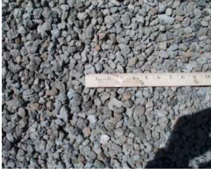
Figure 3.18 Appearance and Maximum Size of Western Aggregate
