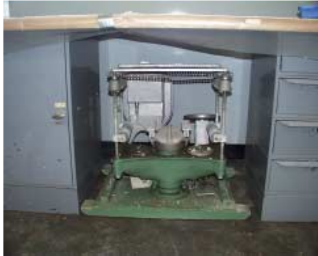
Figure 3.11 Machine Used for Modulus of Rupture Tests
