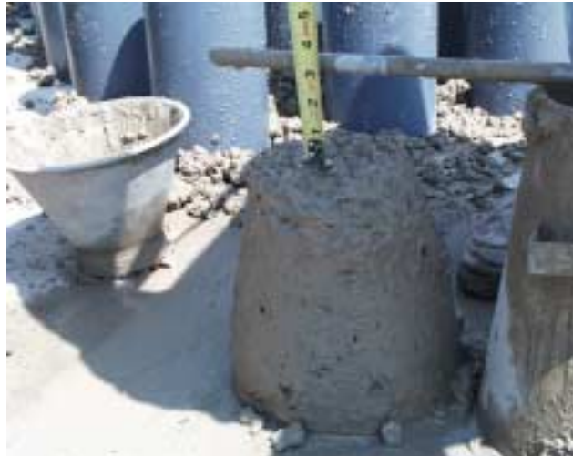
Figure 5.7 Slump for First Batch of 8000 psi Concrete
