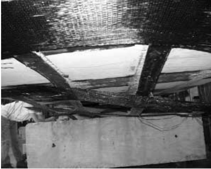
Figure 7.7 Bottom View Toward North End of Specimen FS-1 after CFRP-Plate Debonding
