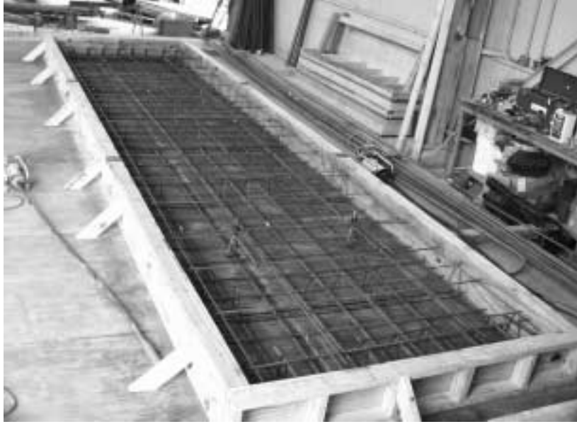
Figure 6.3 Reinforcement in a Typical Flat-Slab Specimen
