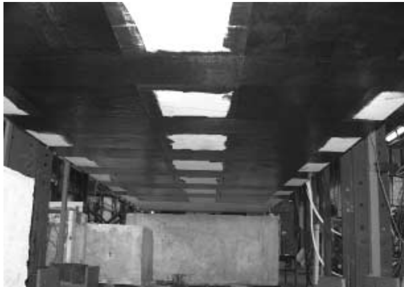
Figure 6.11 Bottom Surface of Specimen FS-2 after Strengthening with the CFRP Wet-Layup System
