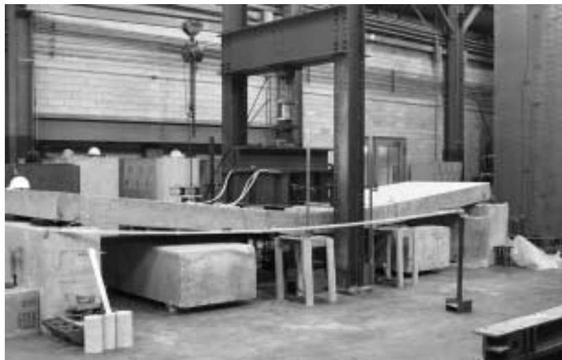
Figure 7.16 West Side of Specimen FS-2 at Deformation Corresponding to Initiation of Concrete Crushing
