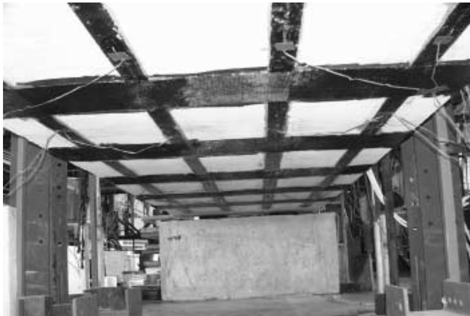
Figure 6.8 Bottom Surface of Specimen FS-1 after Strengthening with the CFRP Pultruded System
