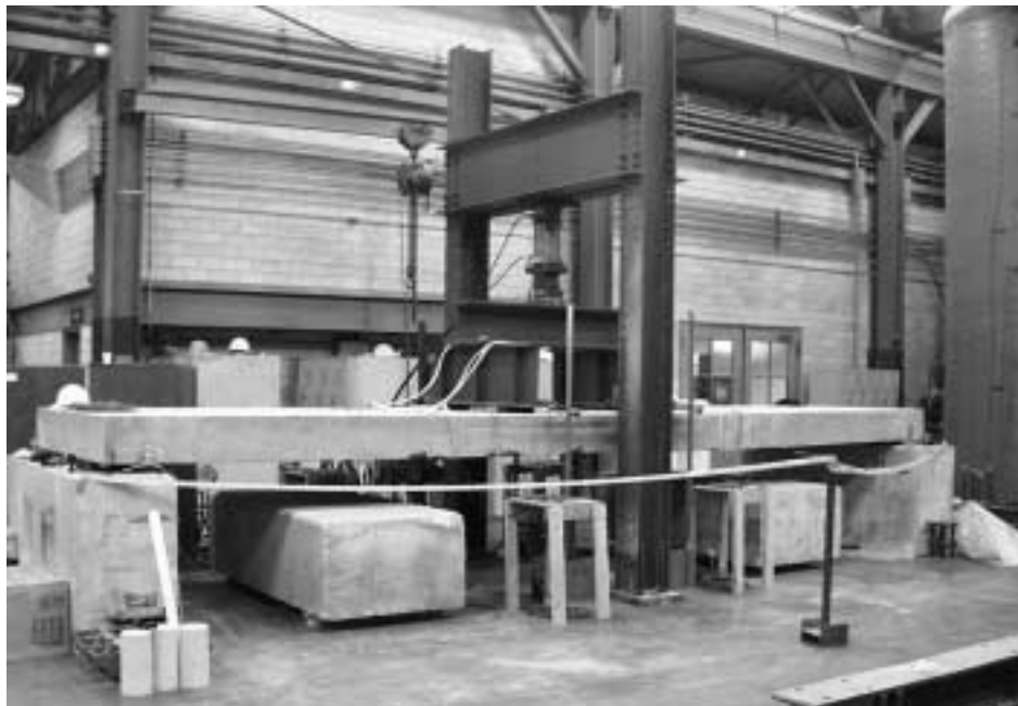
Figure 7.1 Experimental Setup Used for the Laboratory Tests of the Flat-Slab Specimens
