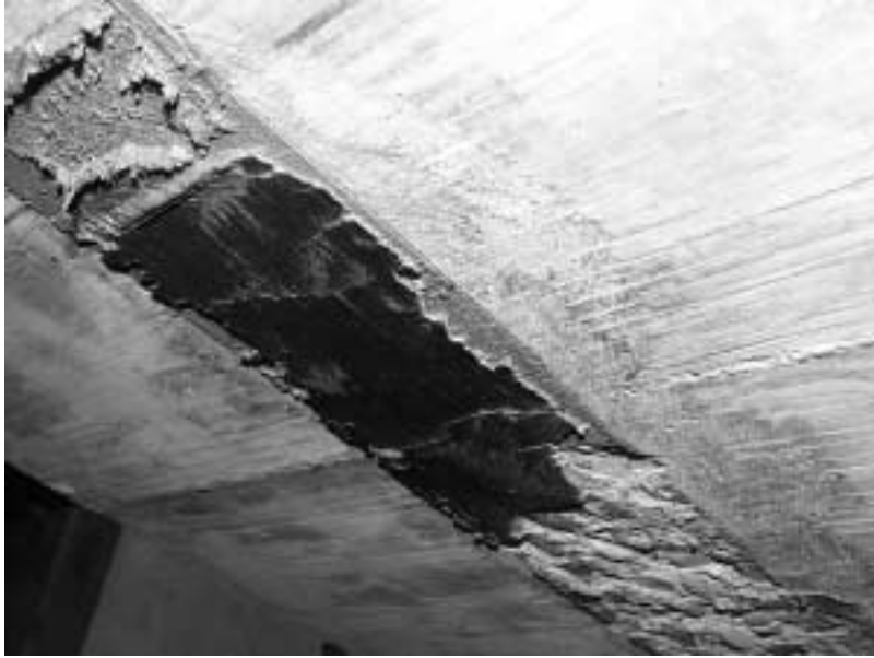
Figure 7.9 Evidence of Plate Delamination of the East CFRP Plate at the North End of Specimen FS-1
