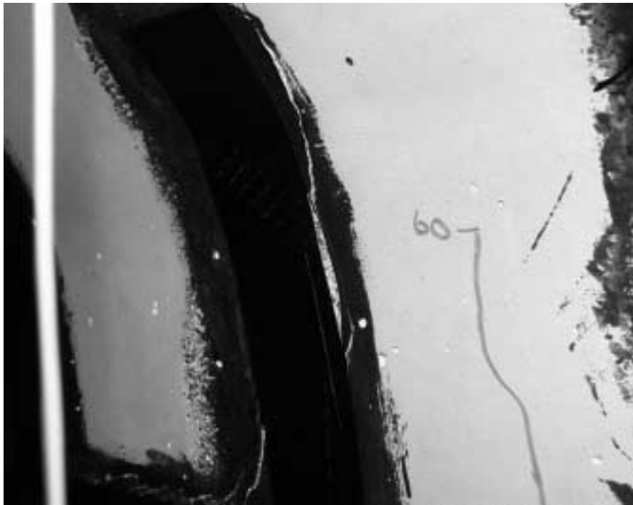
Figure 4.12 Crack Propagation Behind Strap Caused Debonding
