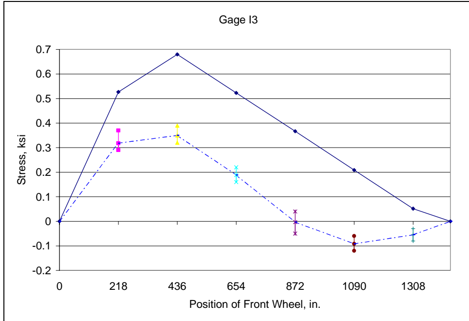
Fig. D.5: Field Test No. 1 - Member L1L2 (Inside) of upstream truss
