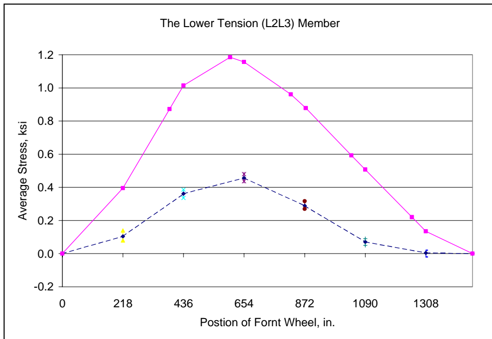
Fig. D.88: Field Test No. 2 - Average stress: Bottom chord (L2L3)
