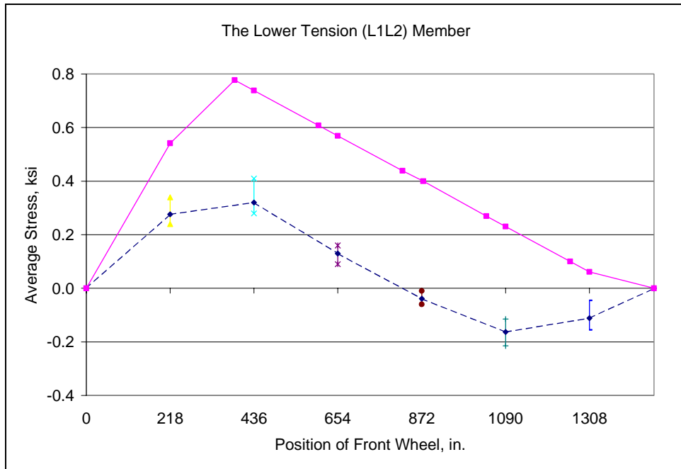
Fig. D.87: Field Test No. 2 - Average stress: Bottom chord (L1L2)
