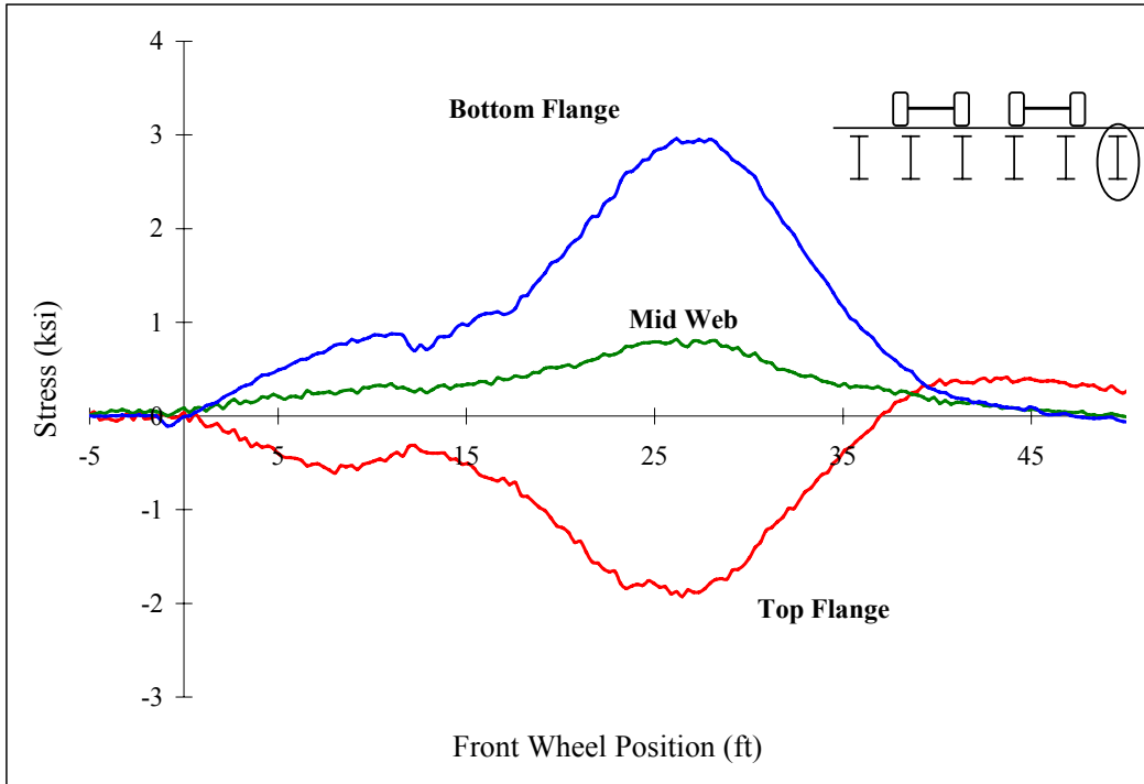
Figure A 4: Midspan stringer 1
