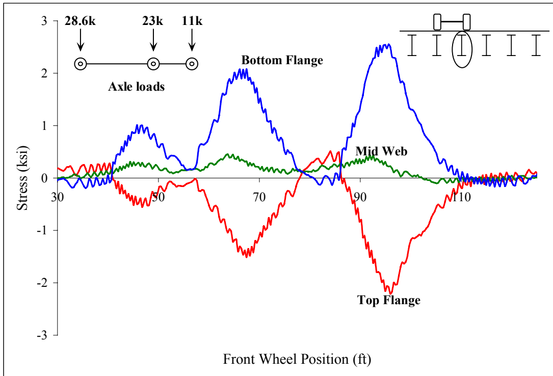
Figure C 5: South quarter point of stringer 3
