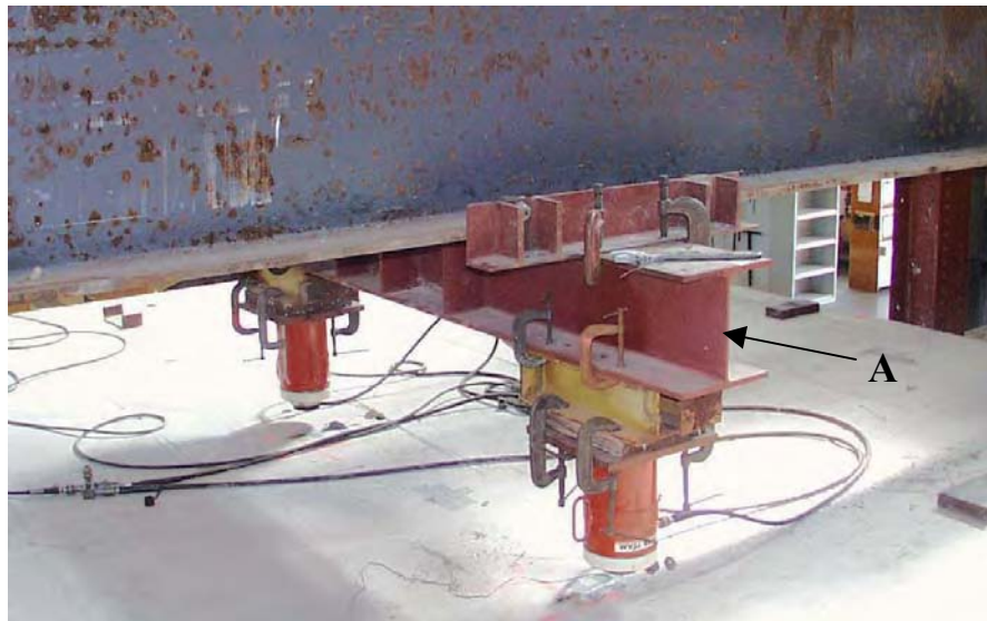
Figure 6.16 Attachment of actuators to load frame
