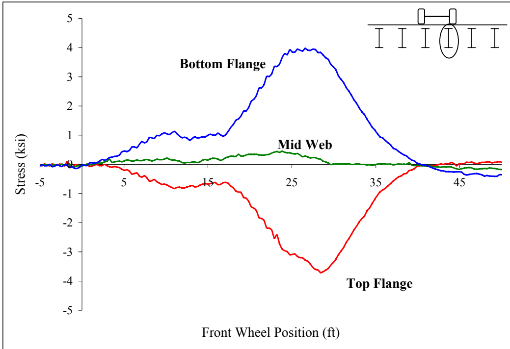
Figure A 16: Midspan stringer 3
