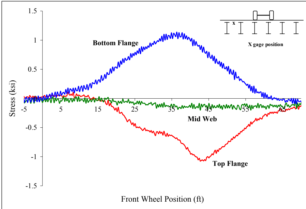
Figure B 40: Beam 2
