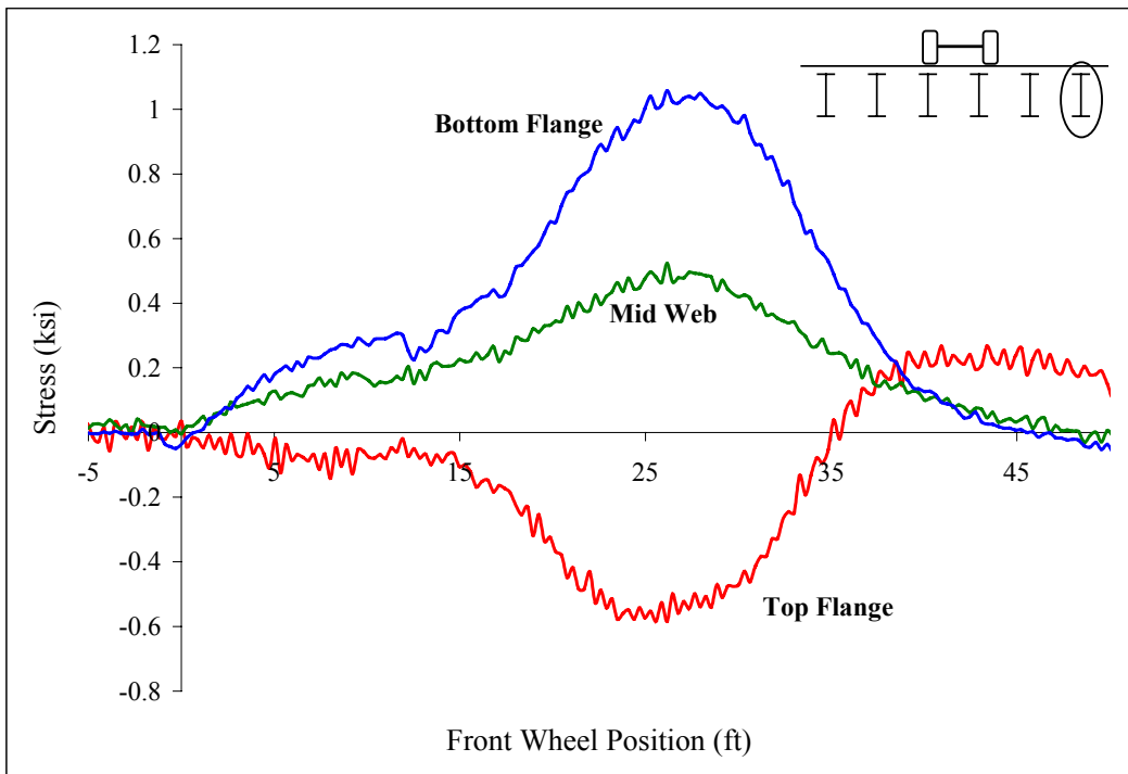
Figure A 31: Midspan stringer 1
