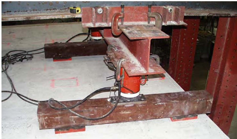
Figure 6.18 Approximation of tandem axle with structural tubing and rubber pads
