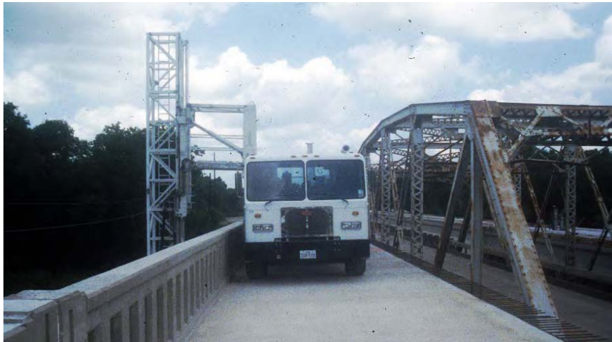
Figure 5.12 TxDOT snooper truck
