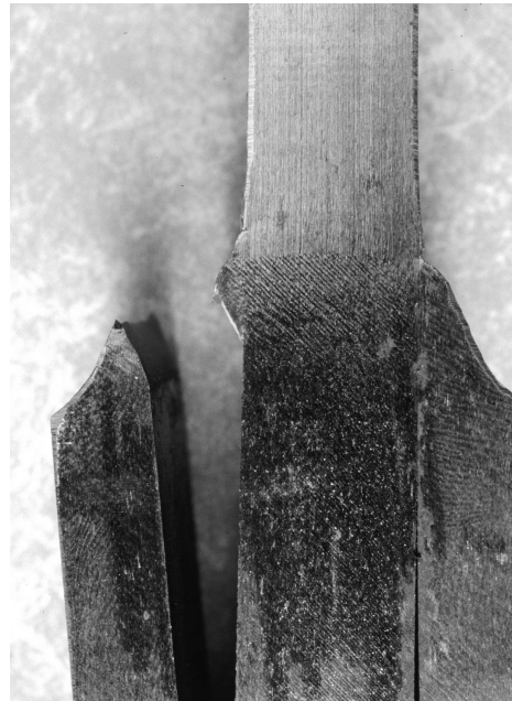
Figure 2.6 Failed weld in tested shear specimen
