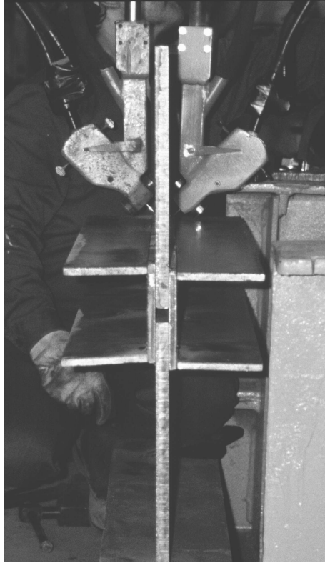
Figure 2.4 Test plate with tacked wing plates
