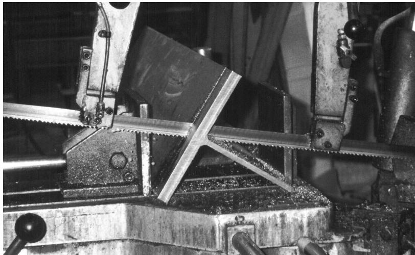
Figure 3.3 Saw-cutting T-bend specimens
