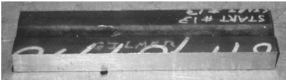
Figure 4.4 Section of WRCVN plate containing weld
