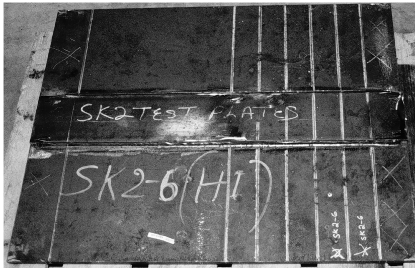
Figure 2.2 Strips marked on test plate
