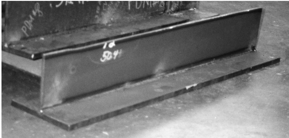
Figure 3.1 T-bend specimens as fabricated
