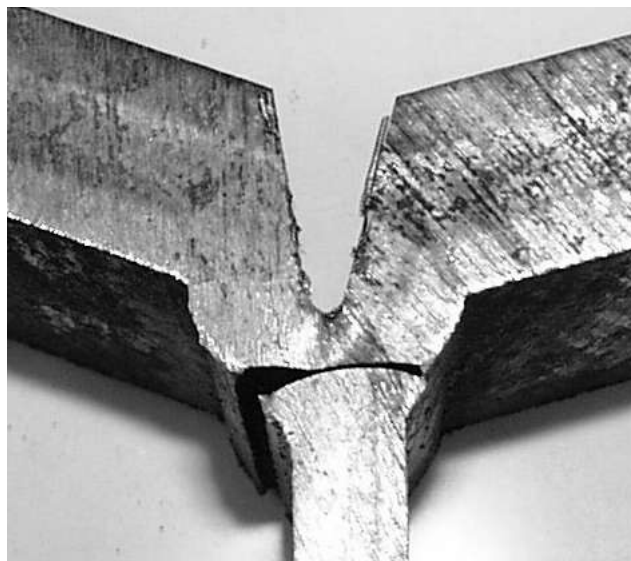
Figure 3.27 Crack in high-heat dart-welded T
