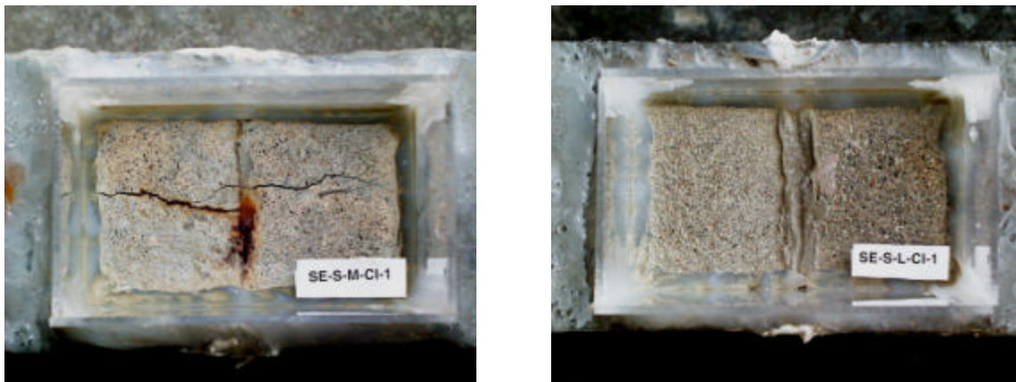
Figure 5.2 Top View of the Effect of a Faulty Epoxy Joint (SE-S-M-CI-1) Compared to a Sound Epoxy Joint (SE-S-L-CI-1).
