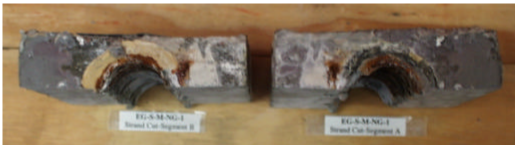
Figure 4.28 Incomplete Epoxy Coverage in Epoxy/Gasket Joint (EG-S-M-NG-1).
