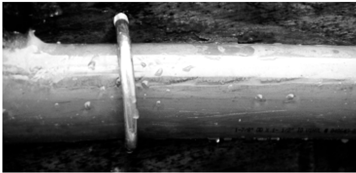
Figure 4.6: Beginning of Void Formation at Intermediate Crest
