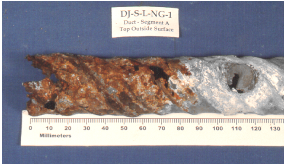
(a) Outside Surface of Duct (joint location at left end)
