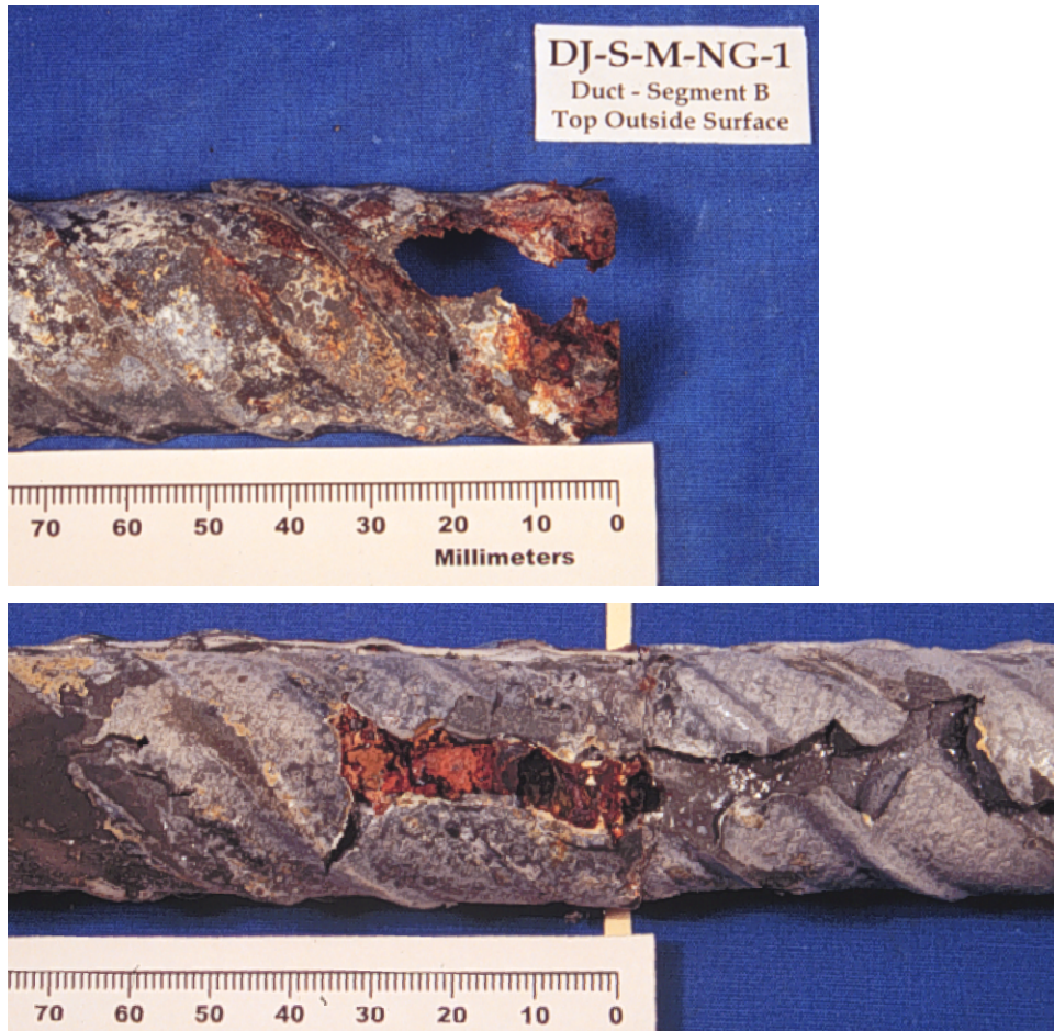
Figure 5.6 – Hole in Duct Corresponding to Grout Void
