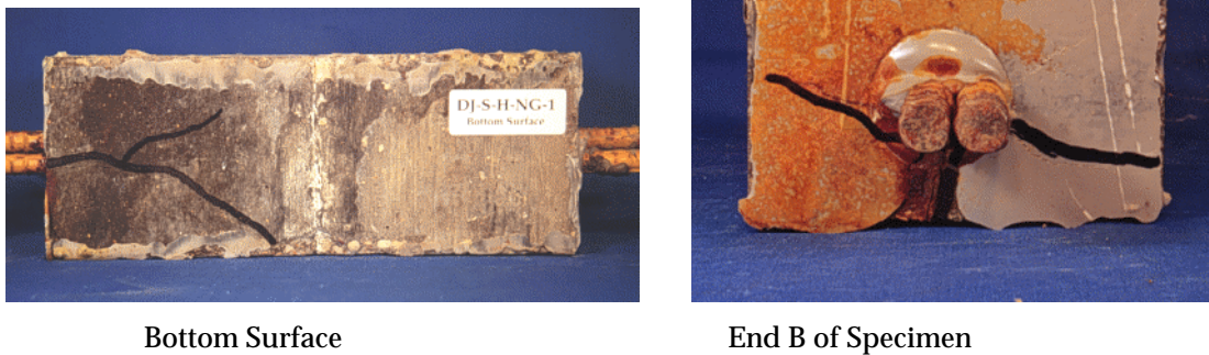
Figure 4.14 – Cracking Due to Rebar Corrosion
