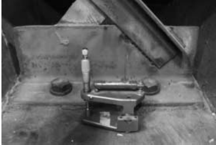
Figure 7.4 Bubble Level at South Support
