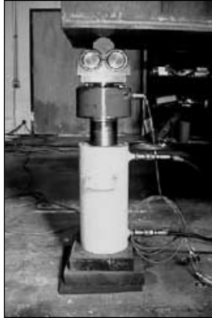
Figure 3.6 Load Ram, Load Cell, and Roller/Bearing Assembly
