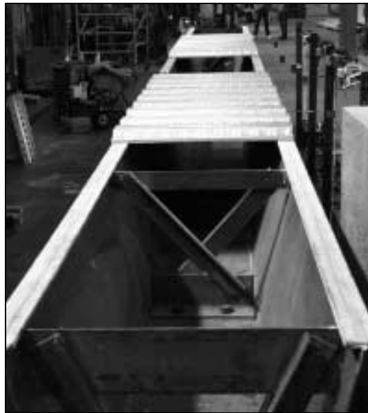
Figure 3.2 Overall Test Setup for Trapezoidal Girder Tests
