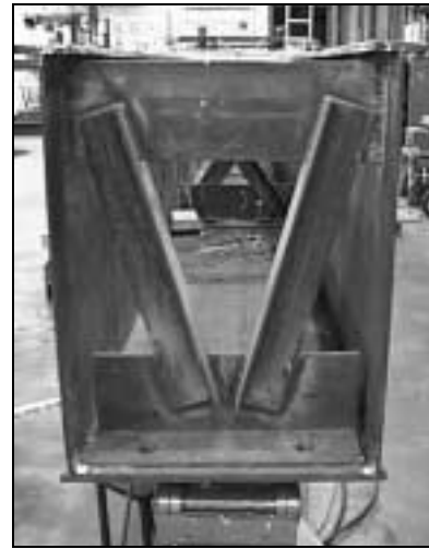
Figure 3.8 K-Brace at Location of Concentrated Load
