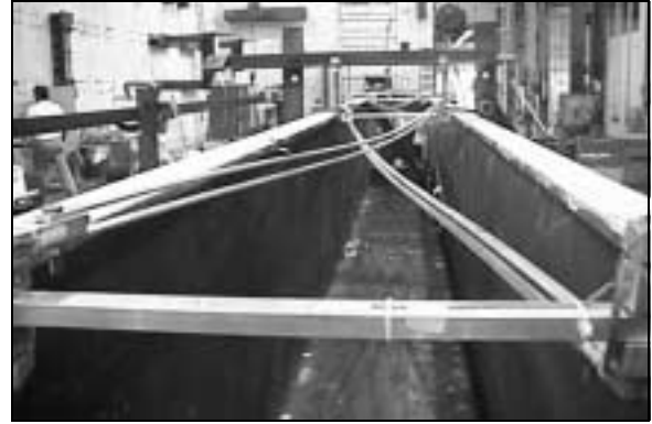
Figure 4.14 Bracing Slack during Initial Loading
