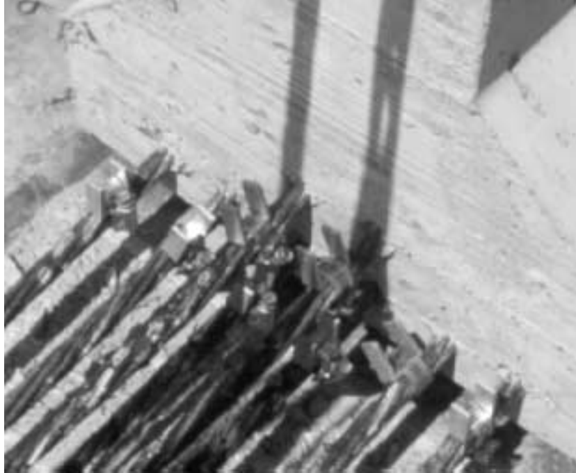
Figure 6.2: Alignment Brackets for Measuring Strand Draw-In
