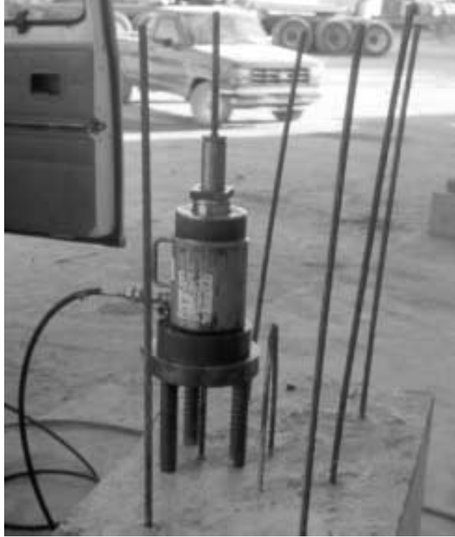
Figure 4.5: Pull-out Test in Progress
