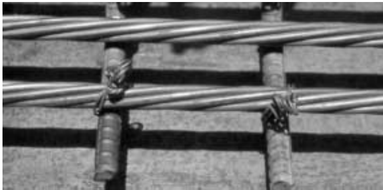
Figure 3.10: "Bright" Strand Surface Condition
