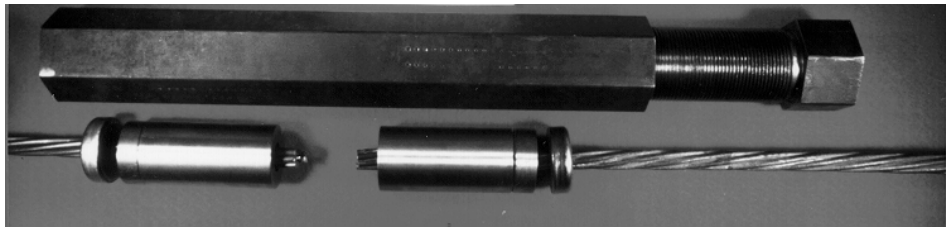
Figure 6-2 Splice hardware designed and used by Alberta Transportation and Utilities Department (fabricated at The University of Texas at Austin)
