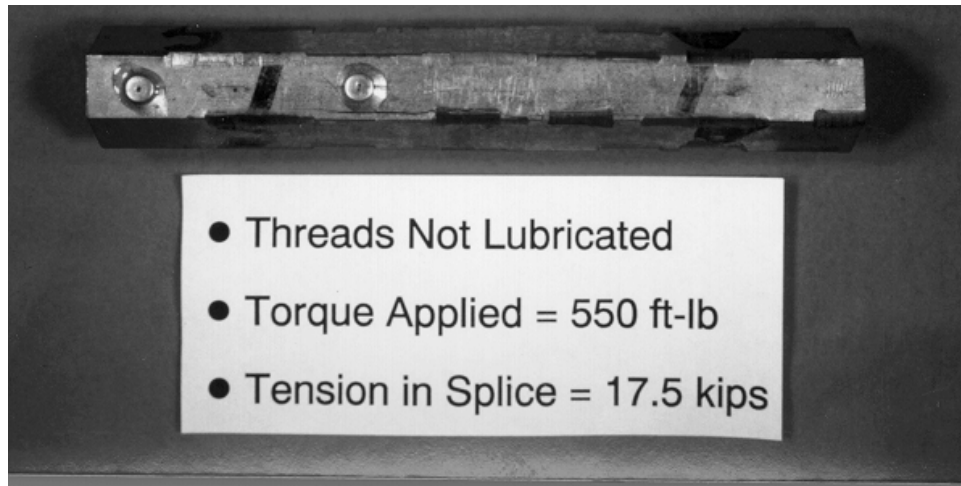
Figure 6-11 Grab-It™ cable splice — exterior of turnbuckle - dry threads - torque proof test
