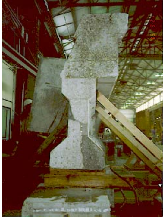
Figure 5- 38 Photograph showing saw-cut section while girder is still in place
