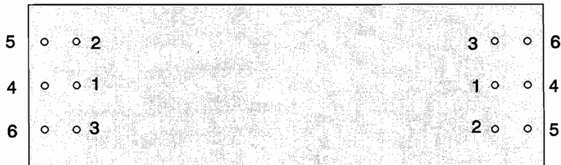
Figure 4.7 Stressing sequence for external vertical post-tensioning bars
