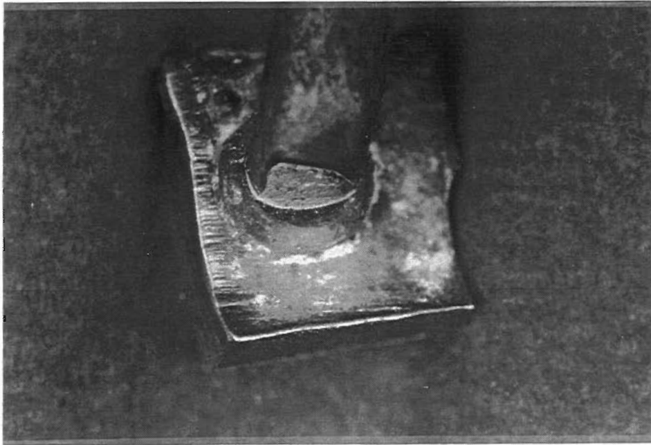
Figure 52 Failure surface of excavated stud
