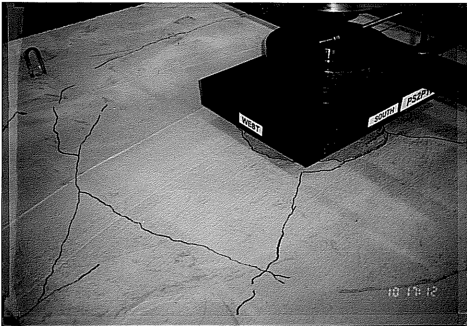
Figure 7.2: Cracking observed on the top surface of precast prestressed panel test specimens after static punching shear failure.
