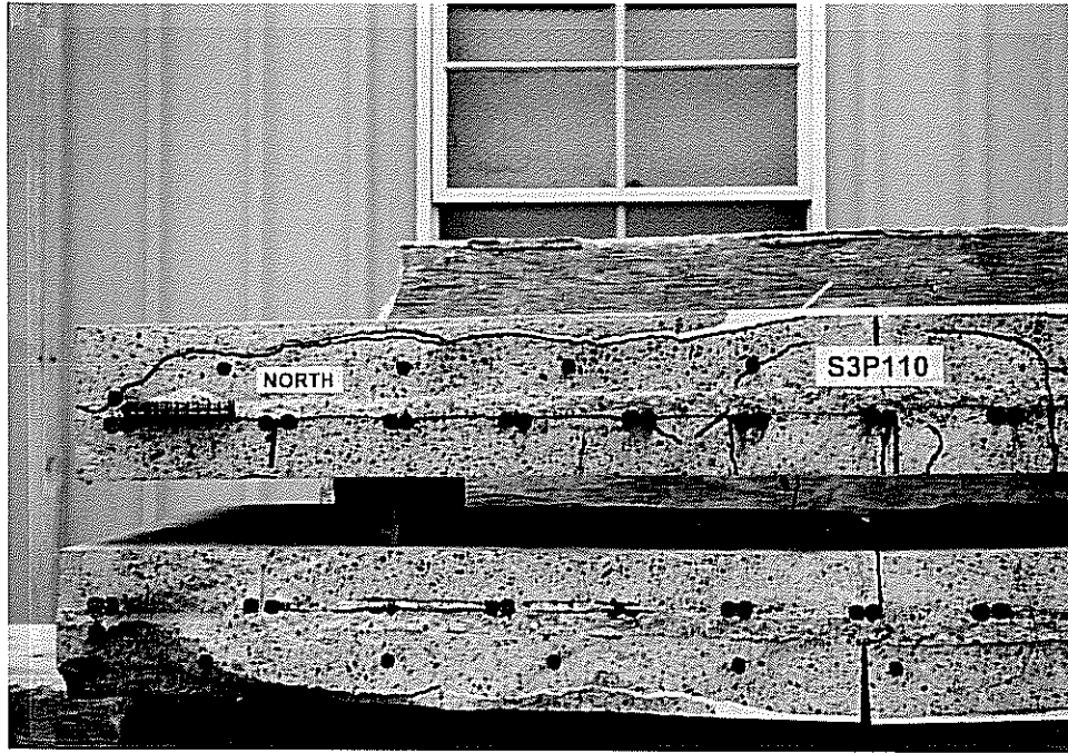
Figure 8.3: Saw cut face (longitudinal section) of cast-in-place pulsating fatigue test Specimen S3P110 (north half).
