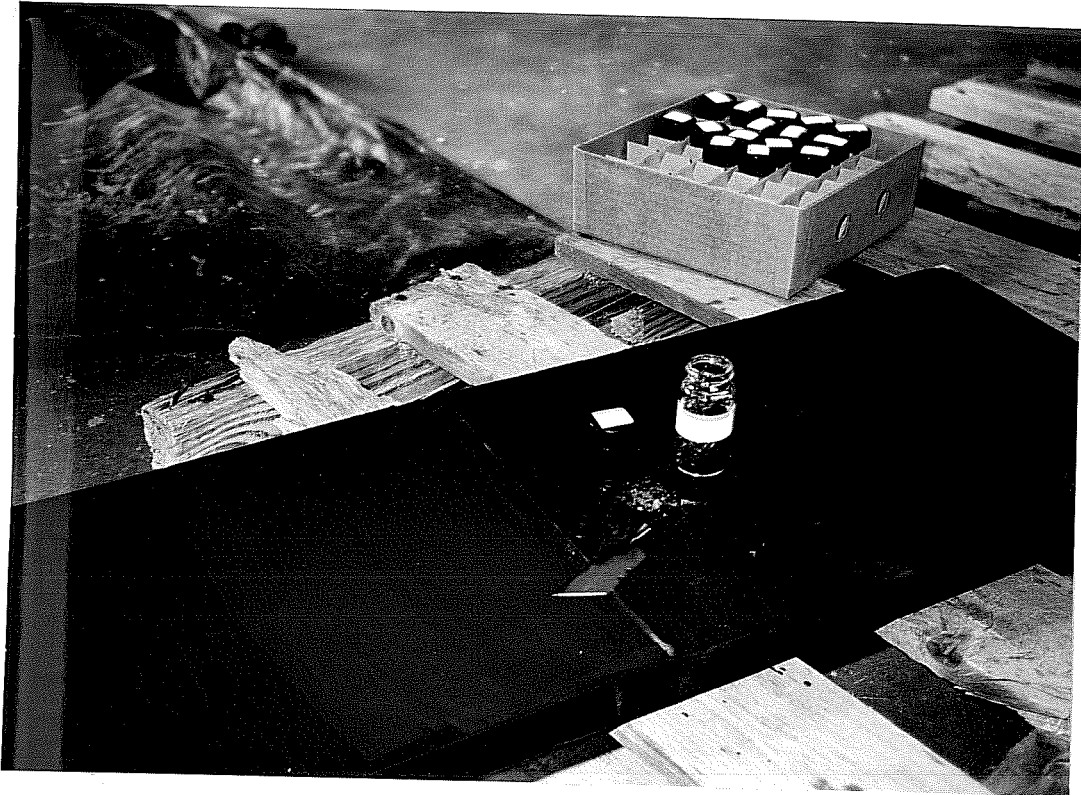
Figure 5- 2 Scraping the bearings with a steel blade and collecting the leachate.
