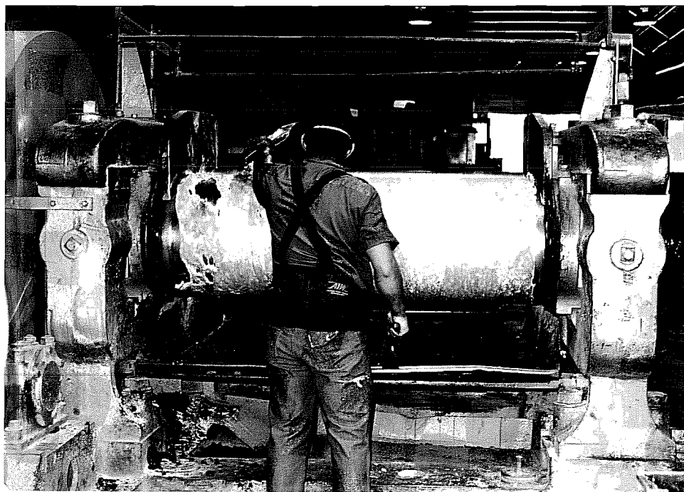
Figure 2- 1 Rubber is worked on the mixing mill
