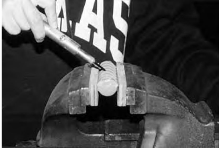
Figure 2.4 Adhesion testing of epoxy-coated bar specimen.
