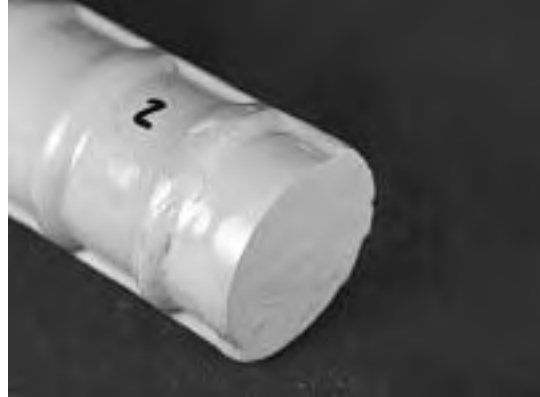
(b) Patched bar end (saw-cut)(II).
