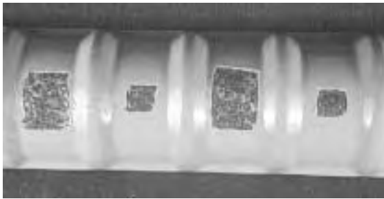
(c) Appearance of damaged areas after two weeks of outside exposure.
