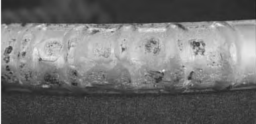
Figure 1.2 Corrosion of patched areas at outside bend on #8 bar with damaged coating greater than 2% (macrocell study).
