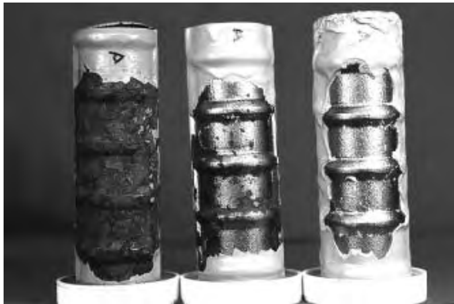
Figure 4.5 Steel surface condition underneath patching materials A , B , and C after 100 days in 3.5% NaCl solution.
