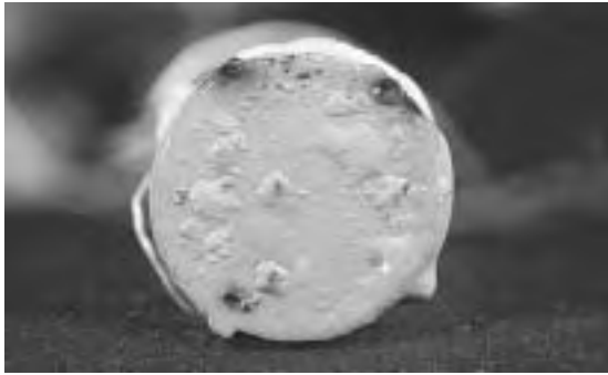
(a) Corrosion stage 1.
