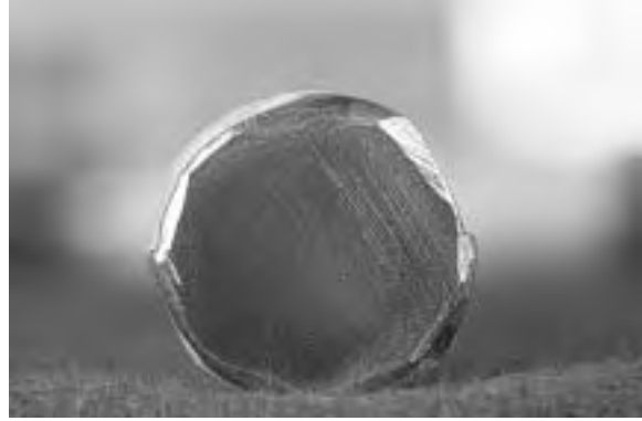
(b) Surface preparation with wheel grinder and wheel brush.
