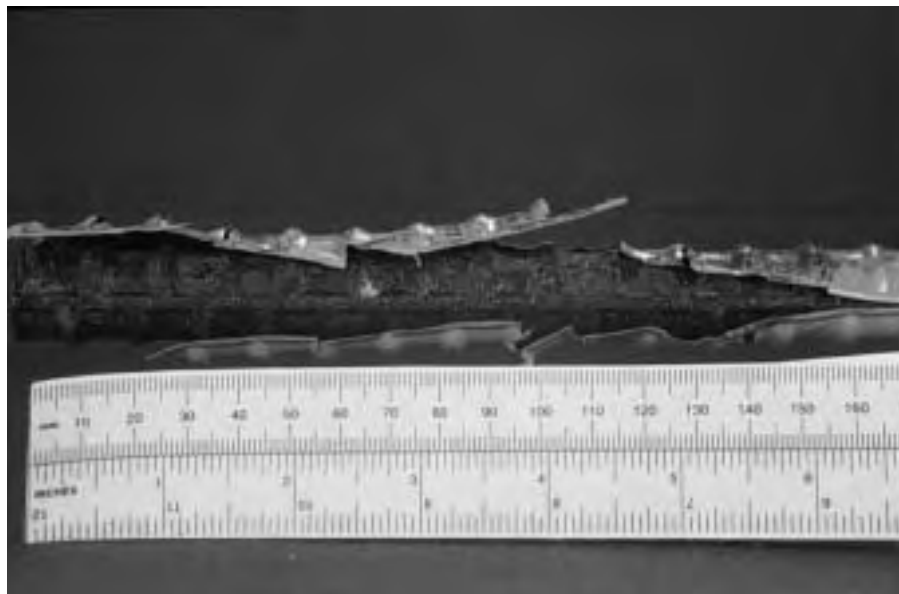
Figure 1.5 Coating debonding with underfilm corrosion of spliced bar within the wetted region after 4.3 years of exposure (beam study).
