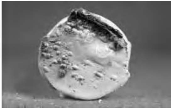
(c) Corrosion stage 3.
