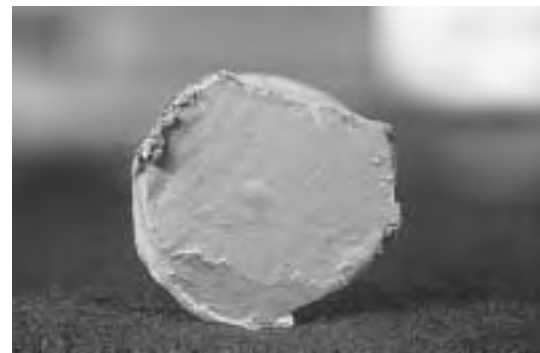
(f) Shear-cut bar end patched by coating applicator (V).
