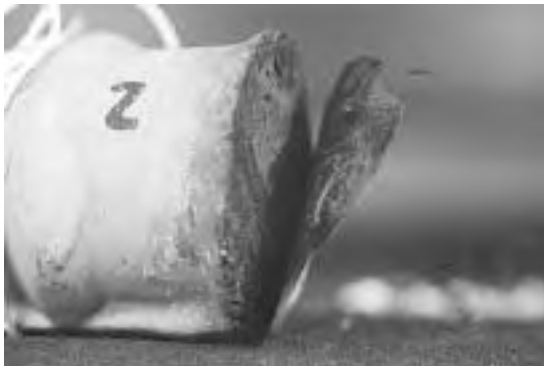
(e) Corrosion stage 4.
