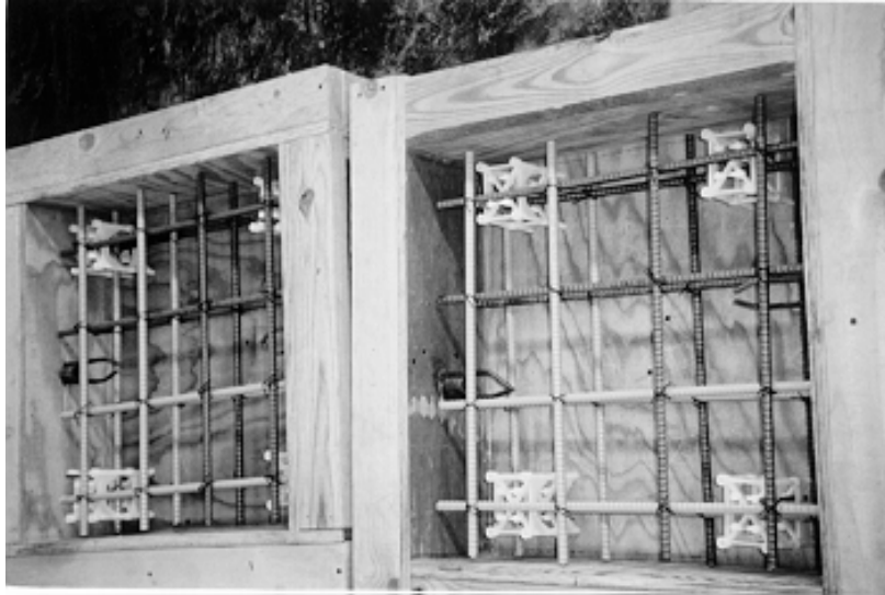
Figure 4.4 Reinforcement of Specimens M8 and R8
