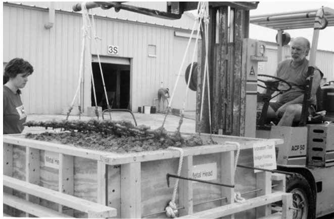
Figure 2.13 Lifting footing reinforcement mat from concrete
