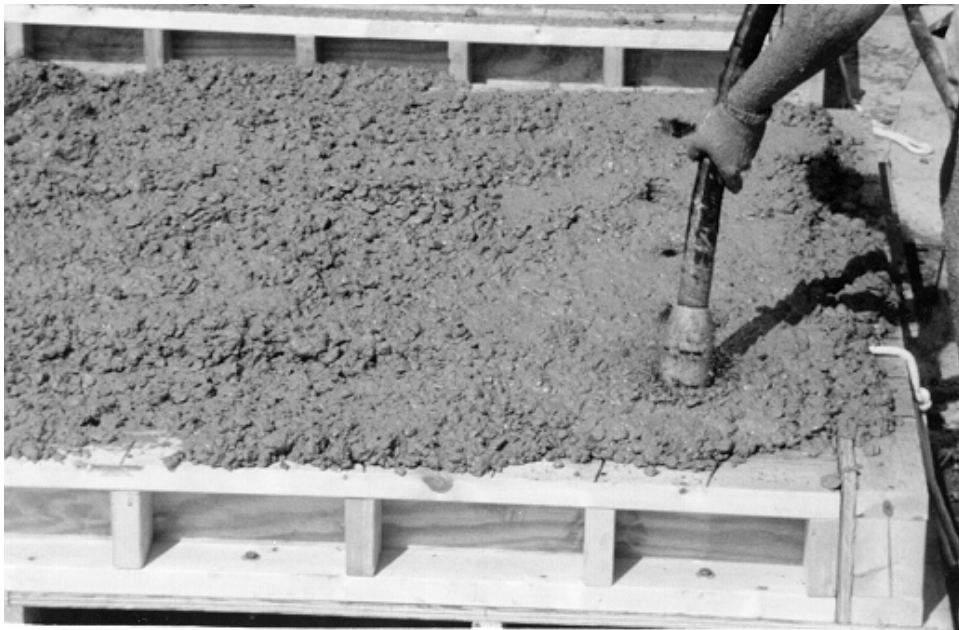
Figure 2. 15 Consolidating slab specimen
