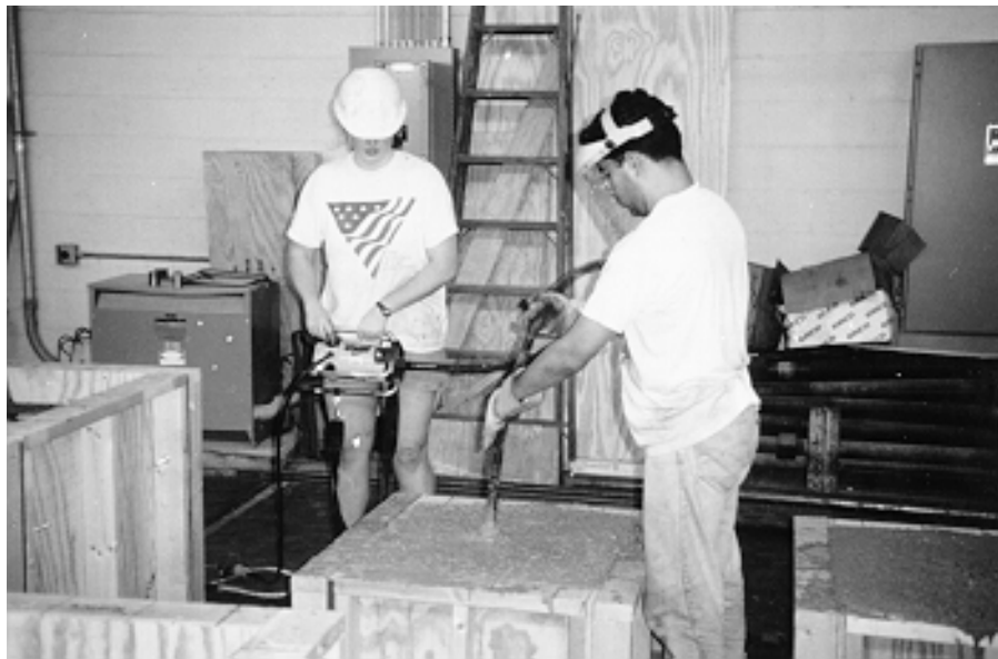
Figure 4. 12 Consolidation of Specimen M17
