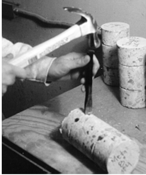
Figure 4. 17 Splitting cores at level of reinforcement
