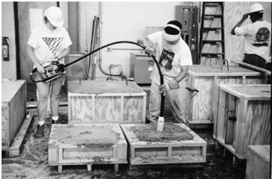
Figure 4. 11 Consolidation of Specimen R8
