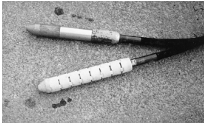
Figure 3.9 Metal (top) and rubber vibrator heads
