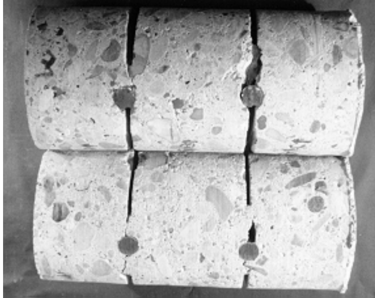
Figure 4. 14 Cores from consolidation test specimens
