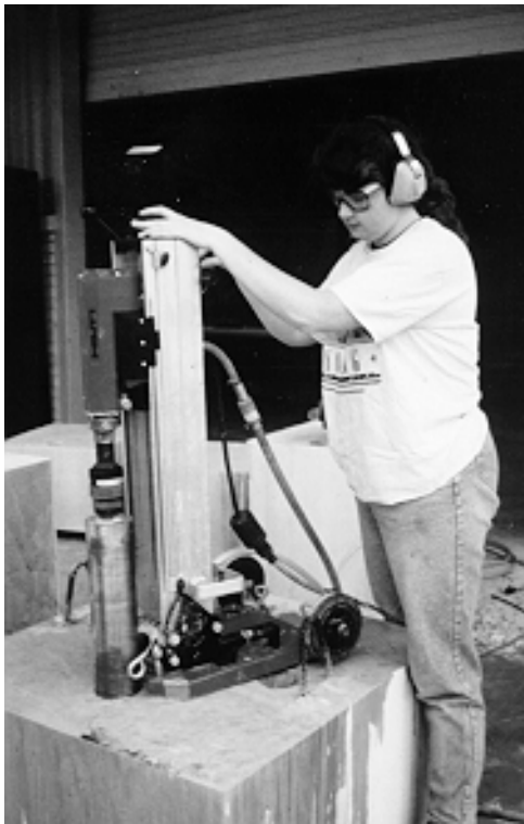
Figure 4. 13 Coring reinforced concrete test specimen
