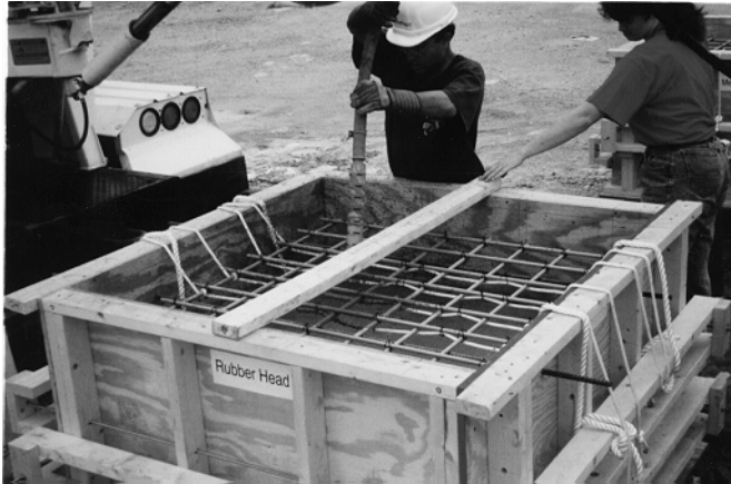
Figure 2.12 Consolidating footing specimen
