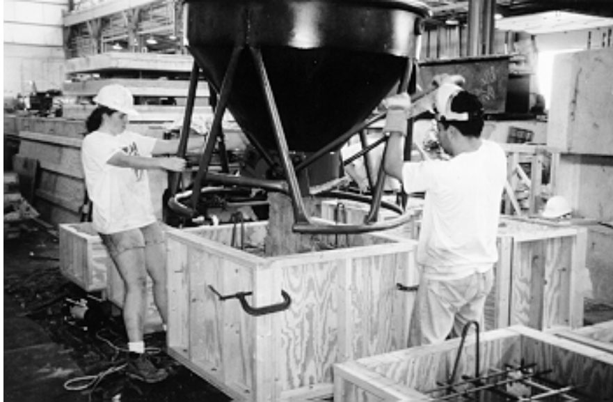
Figure 4. 10 Placing concrete in specimen from overhead bucket
