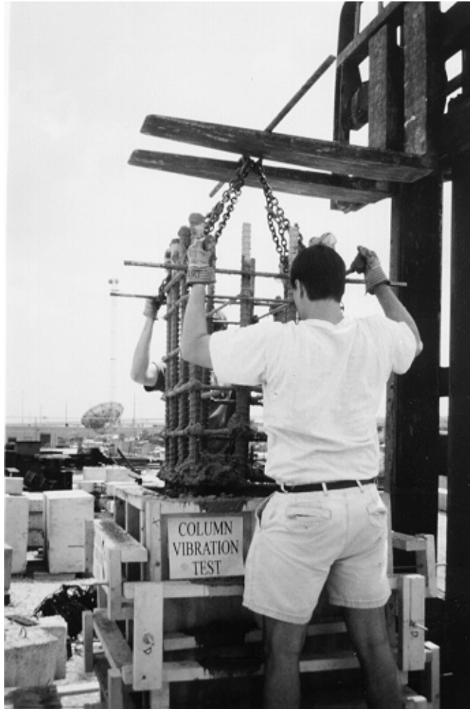
Figure 2.9 Lifting column reinforcement cage from concrete
