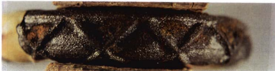
(b) #4 bar with damage area < 2% (A11 group)
