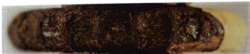
(a) #4 bar with damage area > 2% (A7 group)
