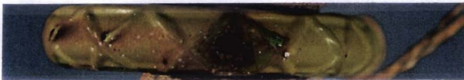
(b) #4 bar with cross deformations (A9 group), few pinholes around and to the left of the patched spot
