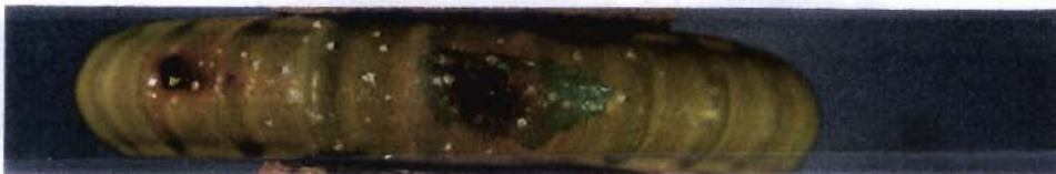
(a) #4 bar with parallel deformations (A2 group), one pinhole to the right of the patched spot
