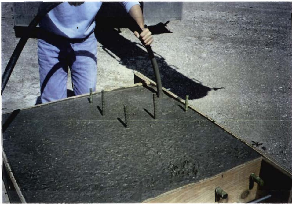
Figure 4.8 Vibration of the column base specimen.
