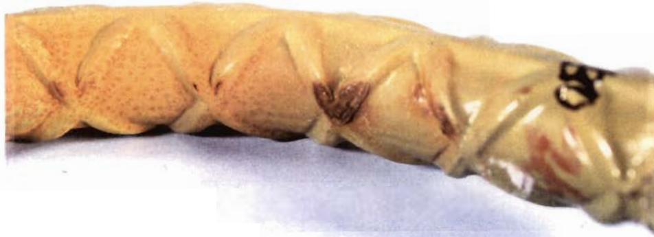
(b) #8 bar with damage area > 2%
