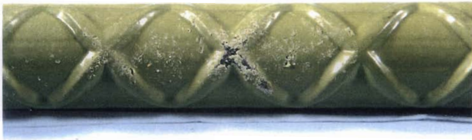
(a) Damage on the lugs
