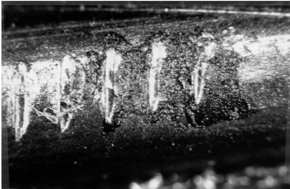
Figure 8- 25 Corrosion between tooth marks on strand
