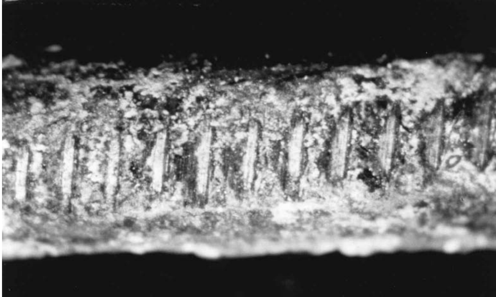
Figure 8- 36 Example of loss of zinc coating
