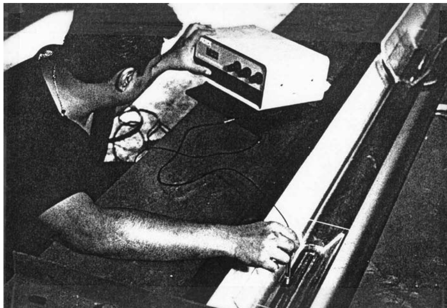
(b) Half-cell potential measurement on "dry" grout surface.
