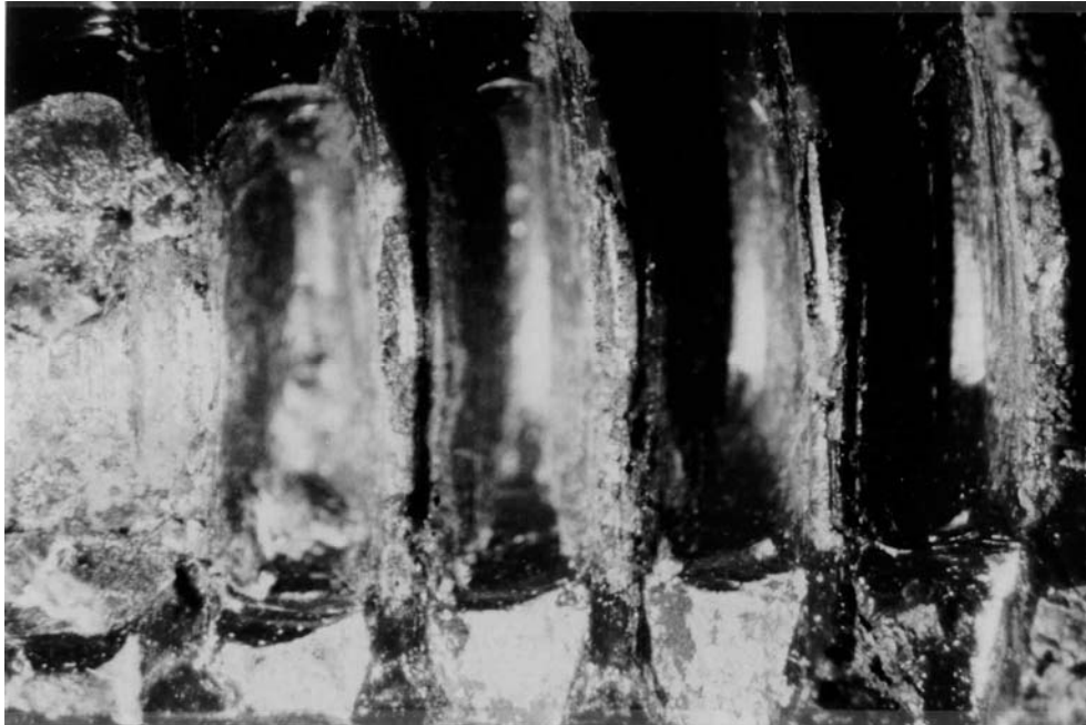
Figure 8-30 Corrosion of strand at tooth mark
