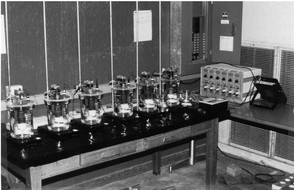
Figure 6-1 Modified accelerated corrosion test method setup
