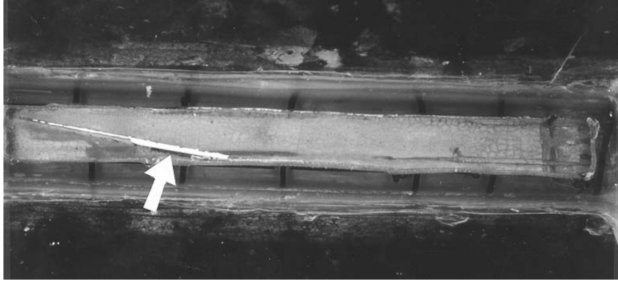
Figure 7- 14 Air trapped adjacent to helical spacer
