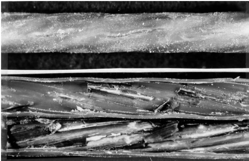
Figure 8- 38 Intrusion of grout into sheathing
