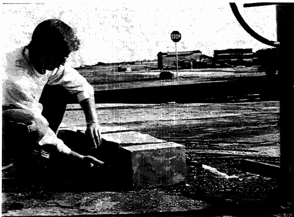
Figure 2.9 Flushing bond test specimen.
