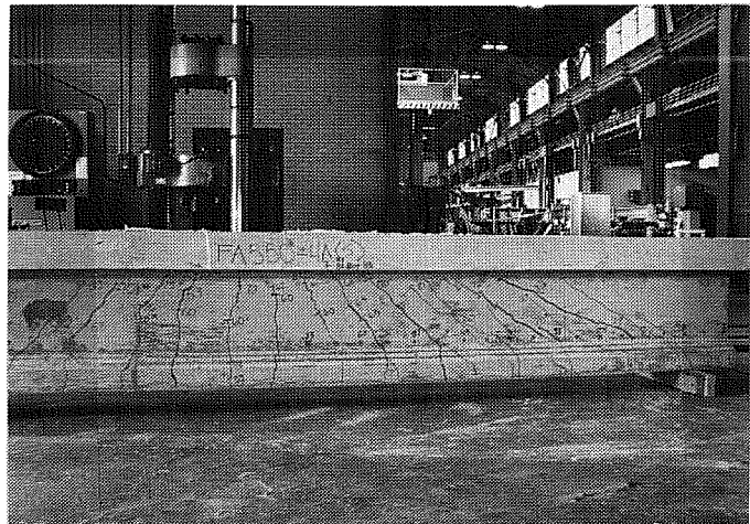
Figure 4.12 Beam FA550-4A: Typical Shear/Bond Failure
