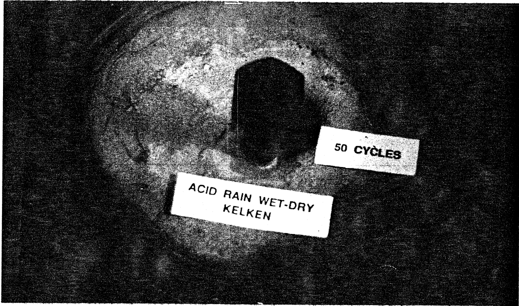
Figure 7.20a Condition of Designation D anchors after 50 cycles of acid rain wetting and drying.
