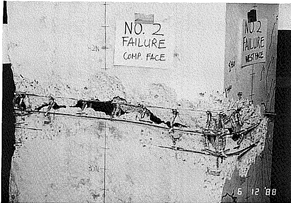
Figure 3.11: Specimen 2M10 Compression Flange Close-Up
