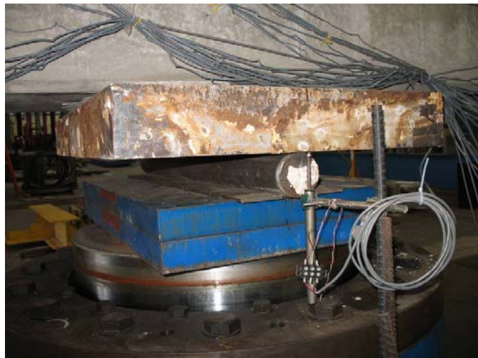
Figure 3.29: Linear potentiometer used to measure the displacement at the load point.
