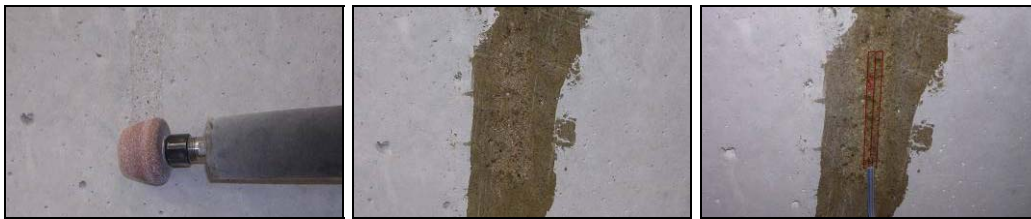
Figure 3.25: Installation of a concrete surface gauge for measuring concrete strains.
