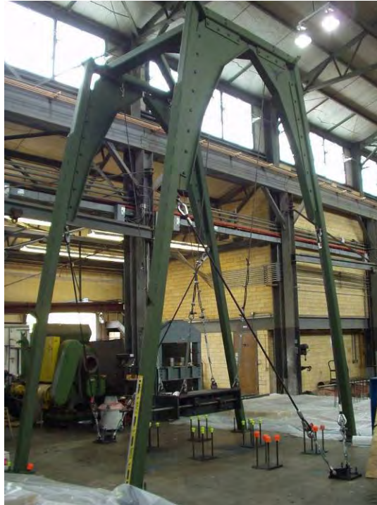
Figure 4.3: Impact test pendulum support frame
