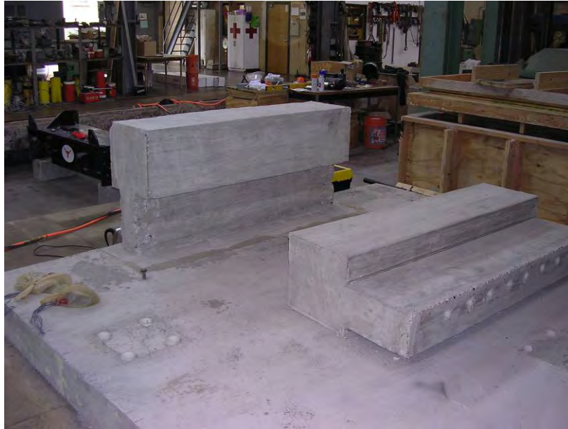
Figure 4.10: Cast-in-place and retrofit T203 bridge barrier specimens
