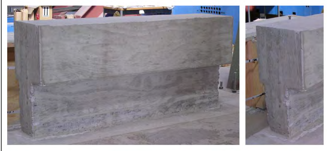
Figure 6.2: Cast-in-place laboratory specimen representing a segment of a TxDOT T203 barrier with continuous base and concrete parapet
