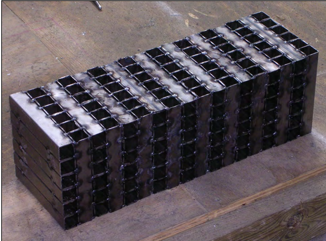
Figure 6.17: Preliminary design of tubular steel crush package
