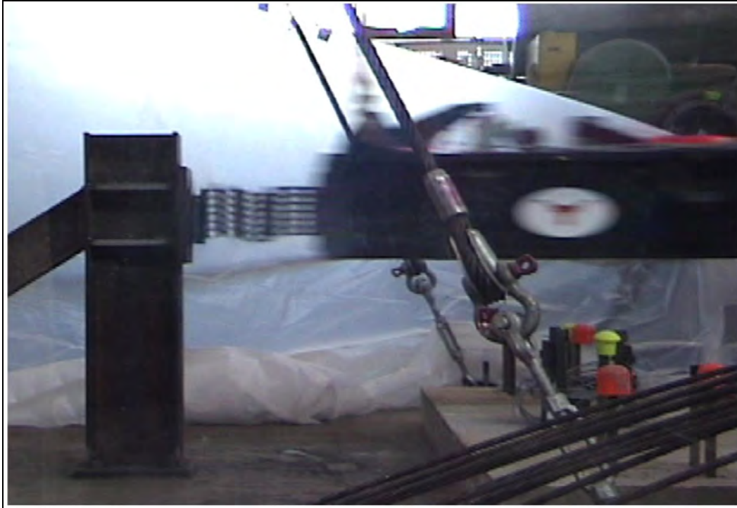
Figure 6.18: Crush package in position on pendulum during a crash test
