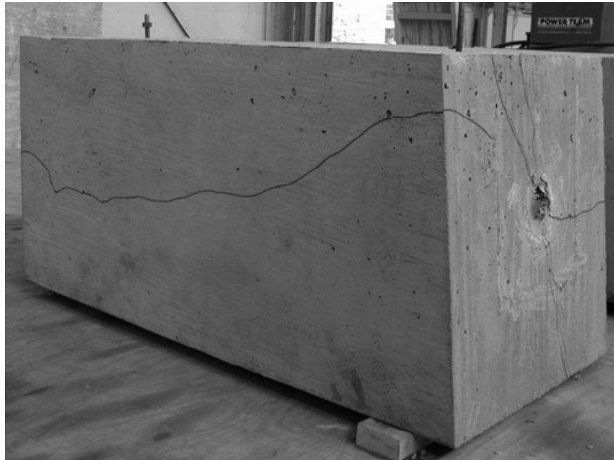
Figure 5-63 Profile 2 of Specimen 0-HD-7.5°-3 after Testing
