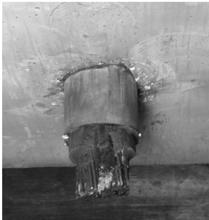
Figure 5-13 Live End of Specimen 1-SP-7.5°-1 after Testing
