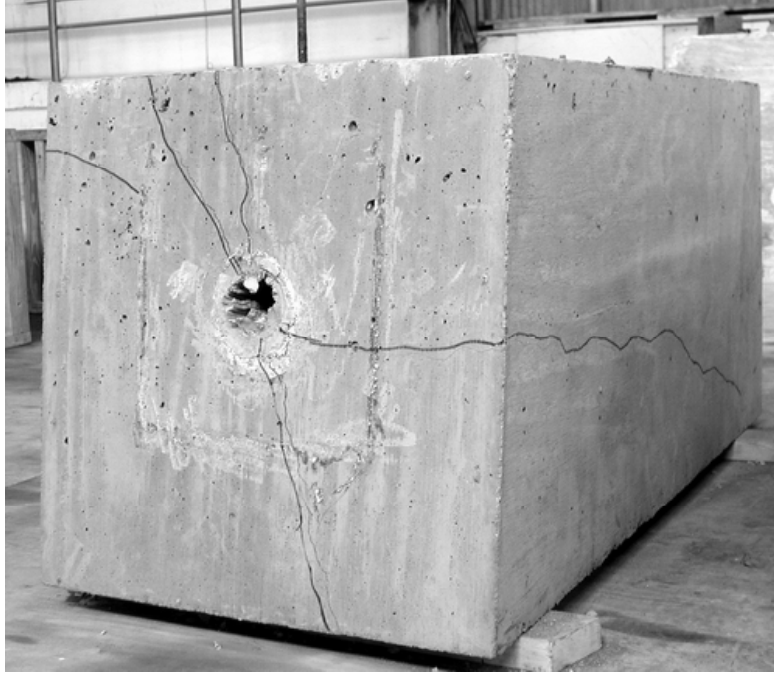
Figure 5-62 Profile of Specimen 0-HD-7.5°-3 after Testing
