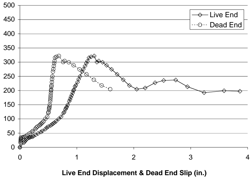
Figure 5-64 Live End Load-Displacement and Dead End Load-Slip Response for Specimen 1-HD-7.5°-1
