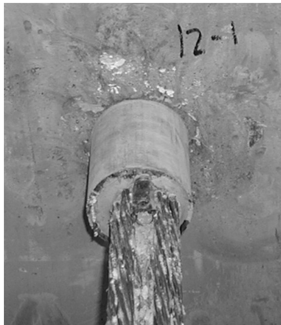
Figure 5-3 Live End of Specimen 0-SP-7.5°-1 after Testing
