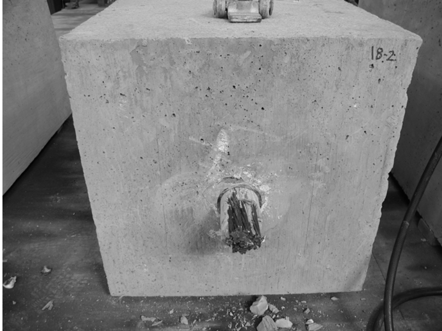
Figure 5-22 Live End of Specimen 2-SP-7.5°-2 after Testing
