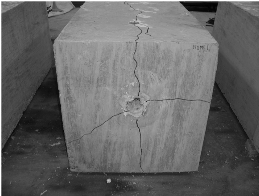
Figure 5-75 Photo of Specimen 2-HD-7.5°-2 after Testing
