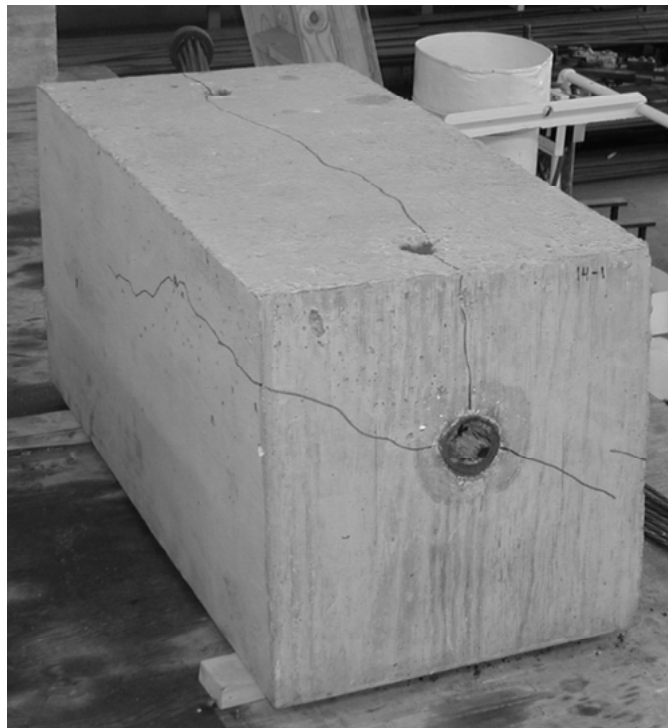
Figure 5-66 Profile of Specimen 1-HD-7.5°-1 after Testing
