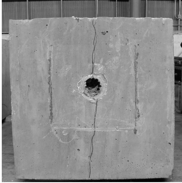
Figure 5-59 Dead End of Specimen 0-HD-7.5°-2 after Testing
