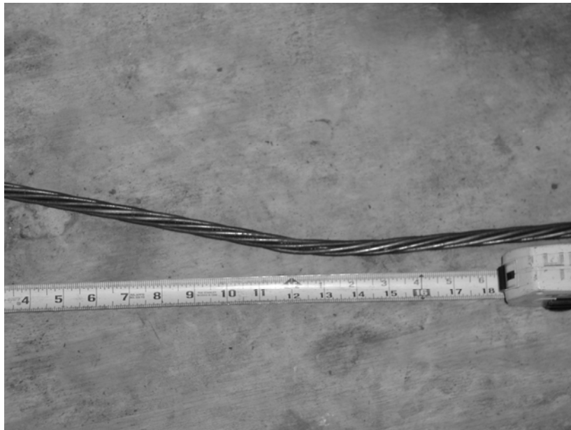
Figure 5-95 Sharp Kink in Strand after Friction Testing
