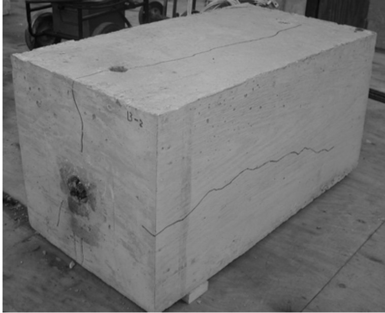
Figure 5-37 Profile of Specimen 1-GD-7.5°-2 after Testing
