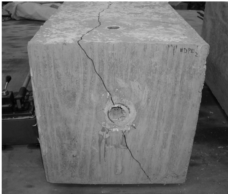
Figure 5-78 Photo of Specimen 2-HD-7.5°-3 after Testing
