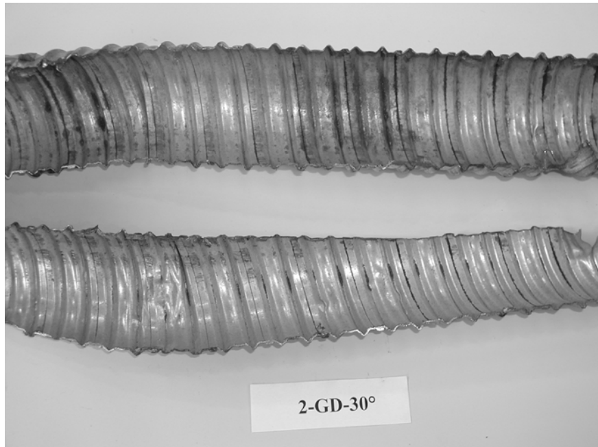
Figure 5-102 Duct from Specimen 2-GD-30° after Testing
