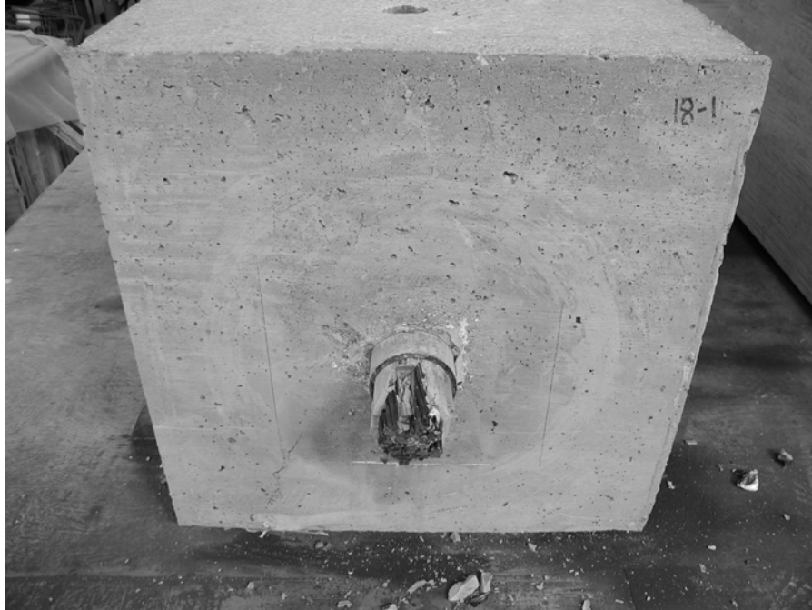
Figure 5-19 Live End of Specimen 2-SP-7.5°-1 after Testing
