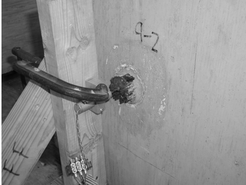
Figure 4-12 Dead End Linear Potentiometer Placement
