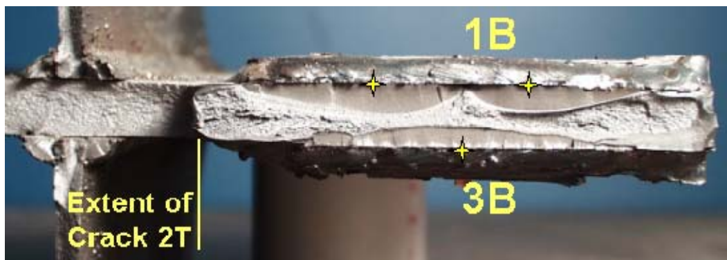
Figure 4-24: 7C-1 Crack at Toe of Welds 1B and 3B
