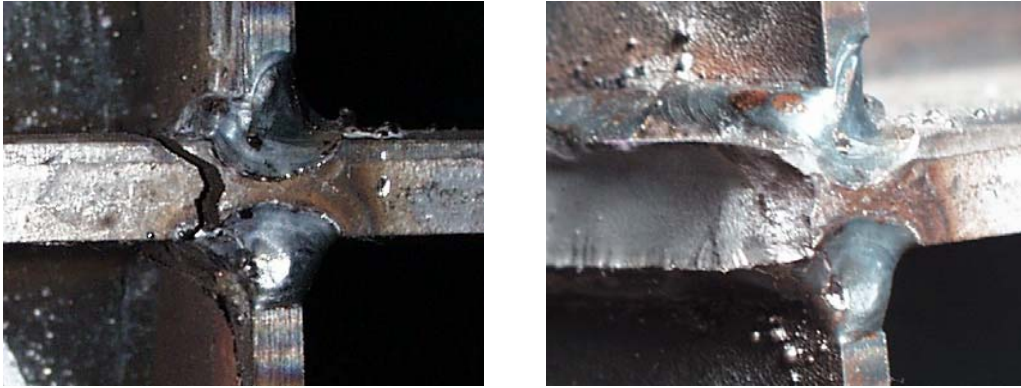
Figure 4-17: Ductile Tear of Flange Edge
