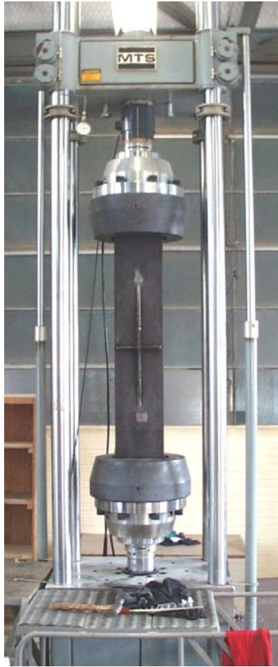
Figure 3-2: MTS Uniaxial Testing Machine with Specimen
