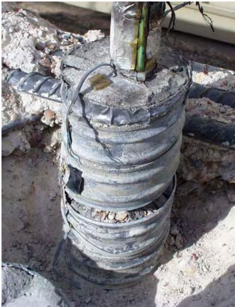
Figure 6.25 Observed Failure of Test 4 (Single Connector, Galvanized Steel Duct)
