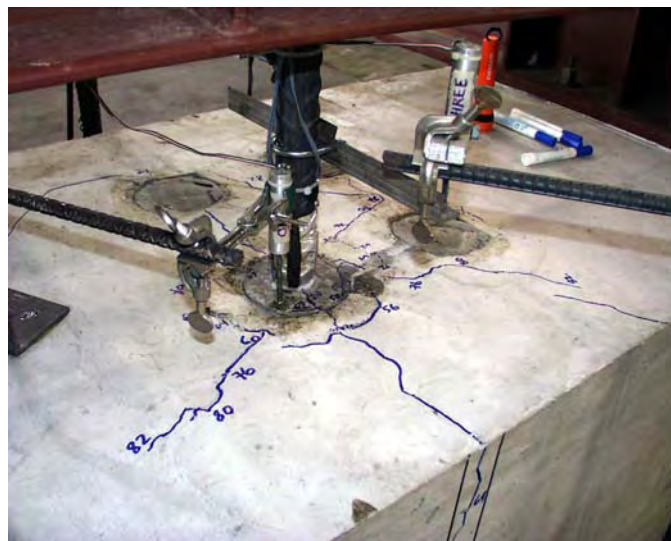
Figure 6.8 Crack Pattern at Failure – Test 9
