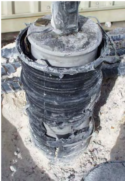
Figure 6.29 Observed Failure of Test 8 (Single Connector, Polyethylene Duct)
