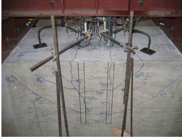
Figure 6.13 Formation of V-Shaped Cracks in Test 32
