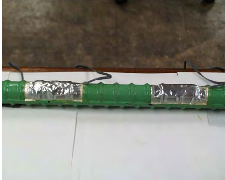
Figure B.3 Two Completed Strain Gage Installations
