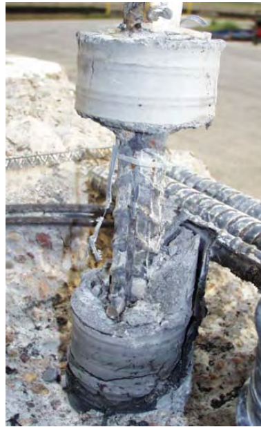
Figure 6.28 Observed Failure of Test 7 (Single Connector, Polyethylene Duct)
