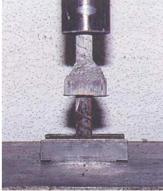
Figure 2.5 Pullout Failure of Generic Grout-Filled Splice Sleeve (Einea et al. 1995)
