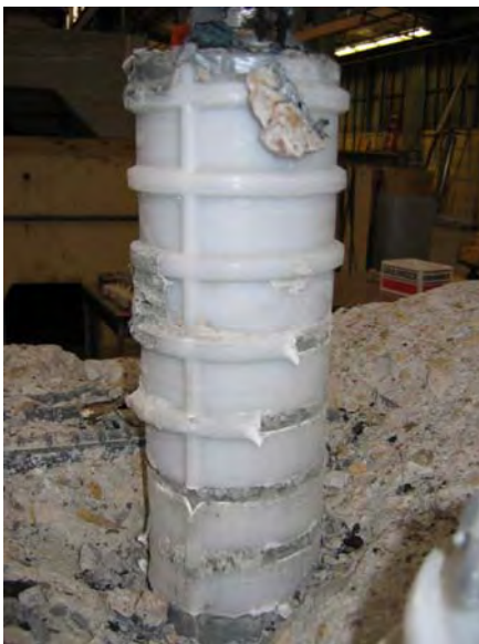
Figure 6.30 Observed Failure of Tests 30 and 28 (Polypropylene Duct)
