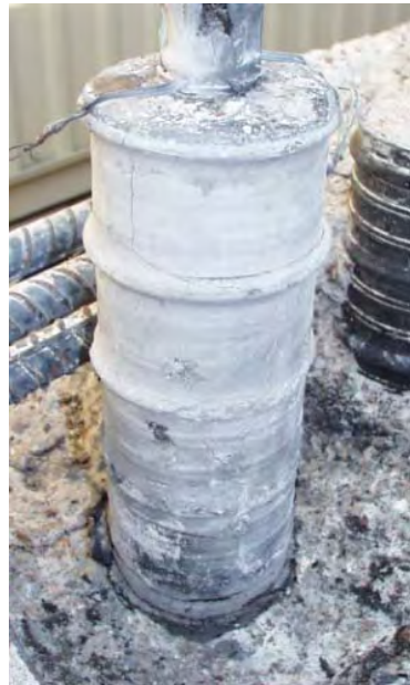
Figure 6.29 Observed Failure of Test 8 (Single Connector, Polyethylene Duct)
