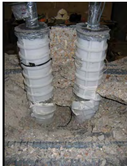
Figure 6.30 Observed Failure of Tests 30 and 28 (Polypropylene Duct)
