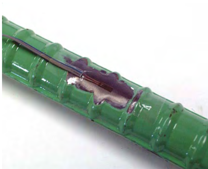
Figure B.1 Surface Preparations on a Connector for Bonding a Strain Gage
