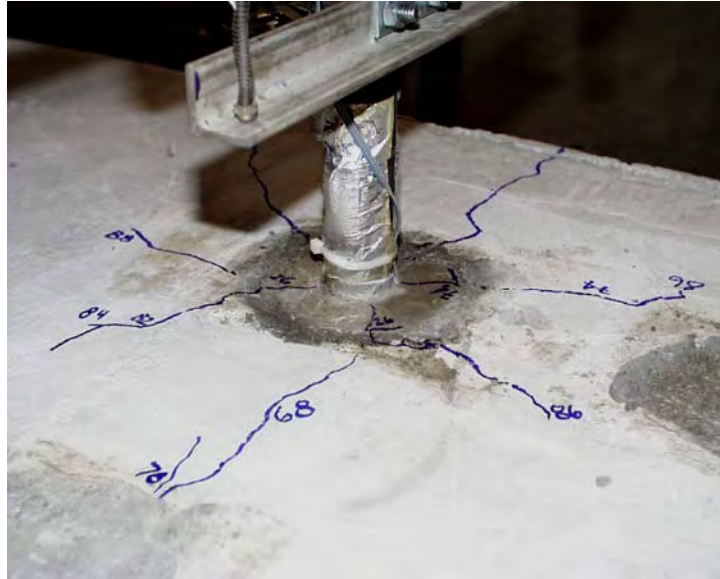
Figure 6.1 Widespread Splitting in Test 10
