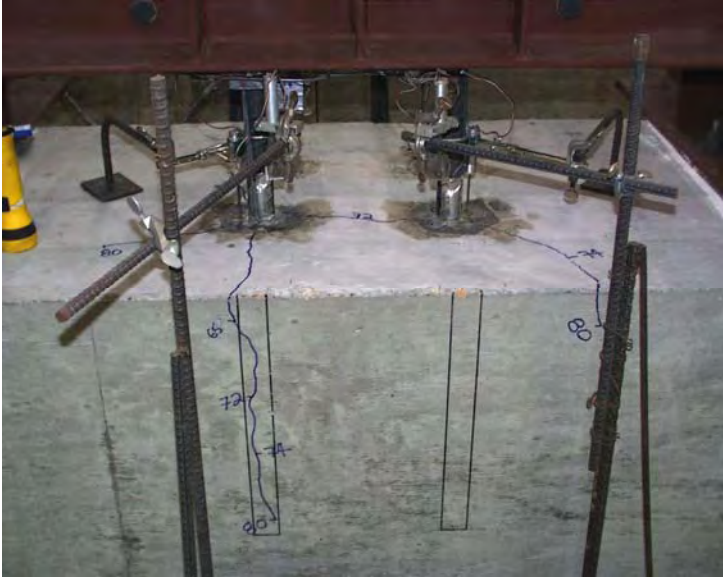
Figure 6.5 Widespread Splitting in Test 23
