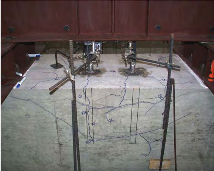
Figure 6.6 Crack Pattern at Failure - Test 23
