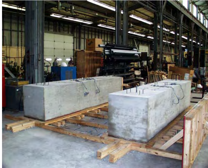
Figure 4.11 Beam Specimens after Formwork Removal
