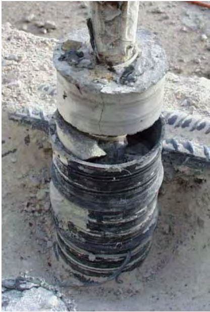
Figure 6.28 Observed Failure of Test 7 (Single Connector, Polyethylene Duct)
