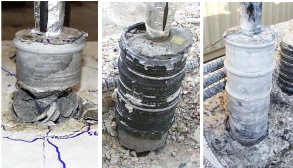
a. Mode 1 Partial Plug Failure without Duct
