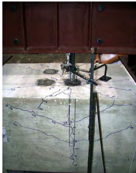
Figure 6.2 Crack Pattern at Failure – Test 10
