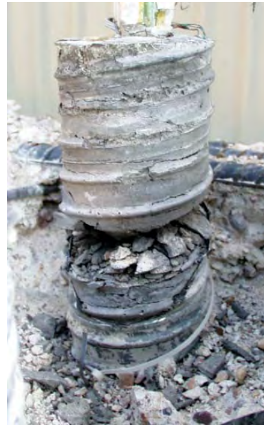
Figure 6.25 Observed Failure of Test 4 (Single Connector, Galvanized Steel Duct)
