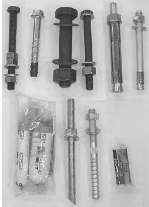
Figure 3.1: Post-installed shear connectors investigated under static loading
