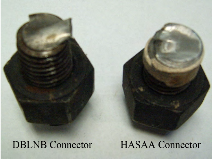
Figure 5.21: Failed sections of shear connectors
