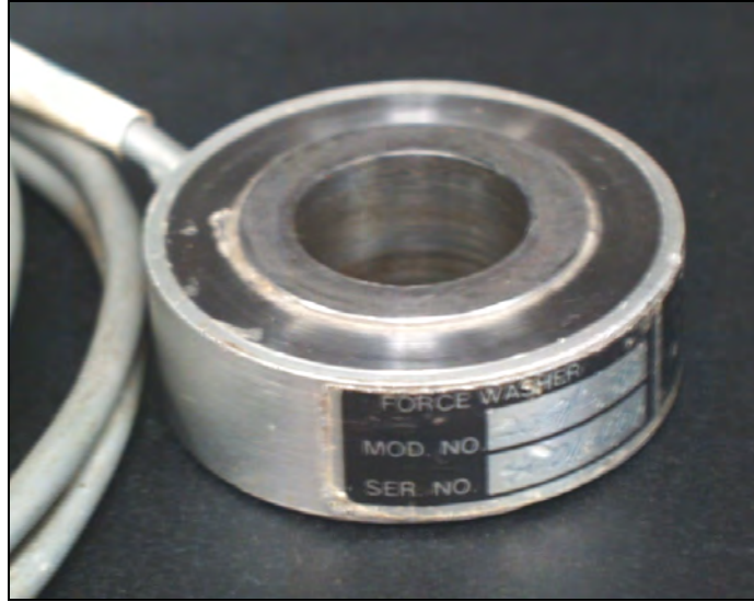
Figure 3.19: Washer load cell
