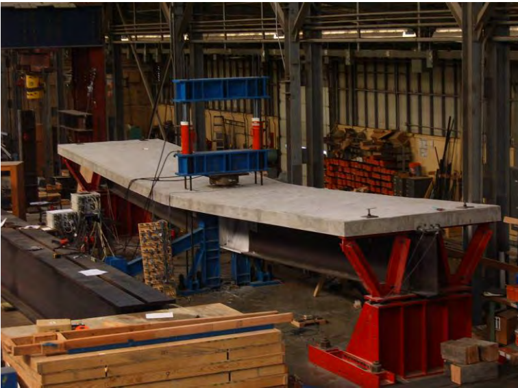
Figure 5.16: Specimen NON-00BS – Overall view of specimen at end of test (11.5-in. deflection)
