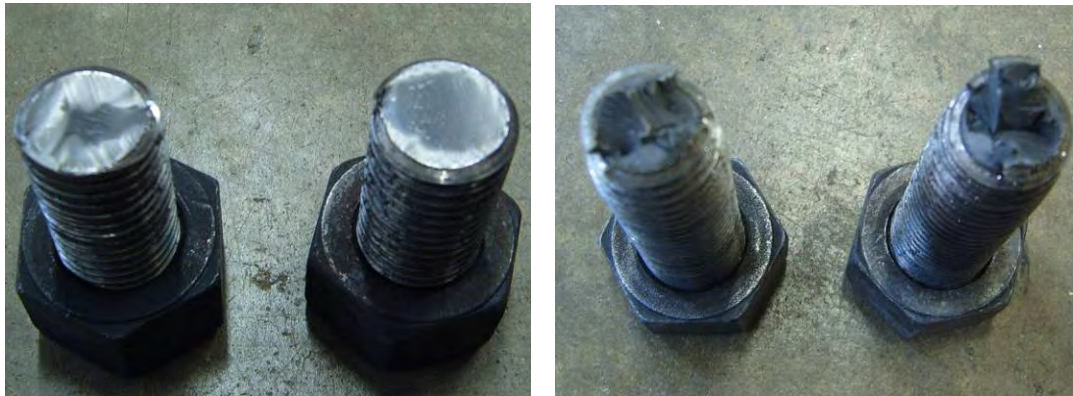
a) Failure sections in shear
