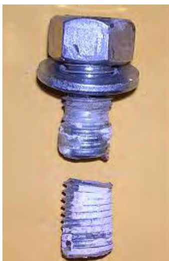
Figure 4.9: HAS-E anchor failed at two locations (Specimen HASAA40)
