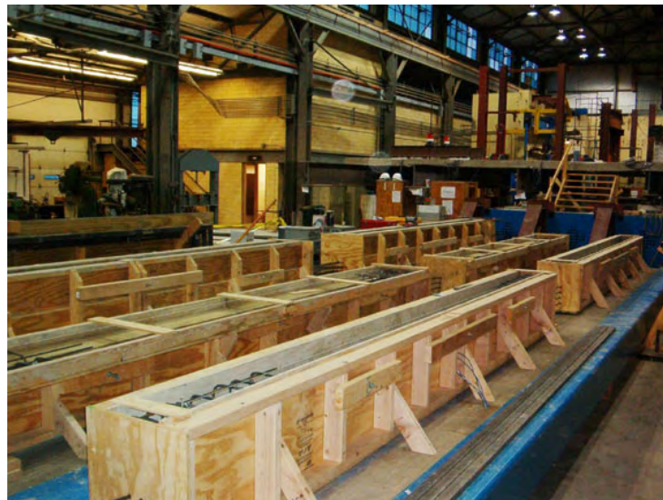
Figure B.2: Prestressing bed at Ferguson Laboratory 2
