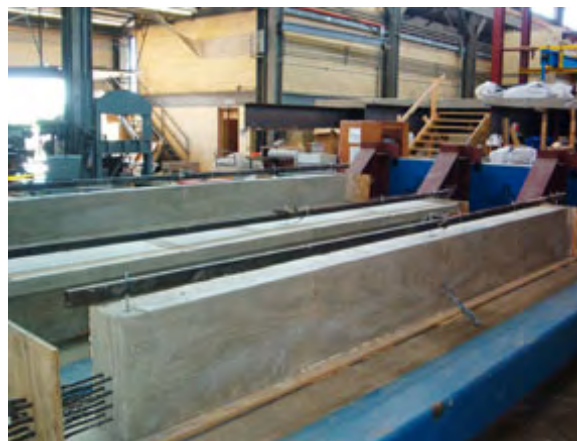
Figure 4-8: Optimized configuration with one potentiometer per beam
