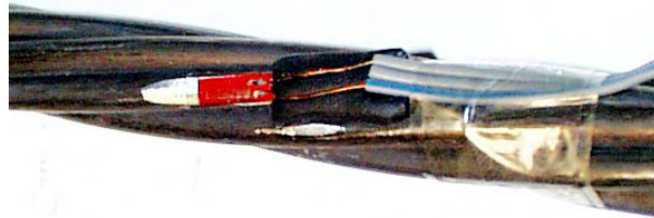
Figure 4-3: Strain gauge mounted parallel to individual wire
