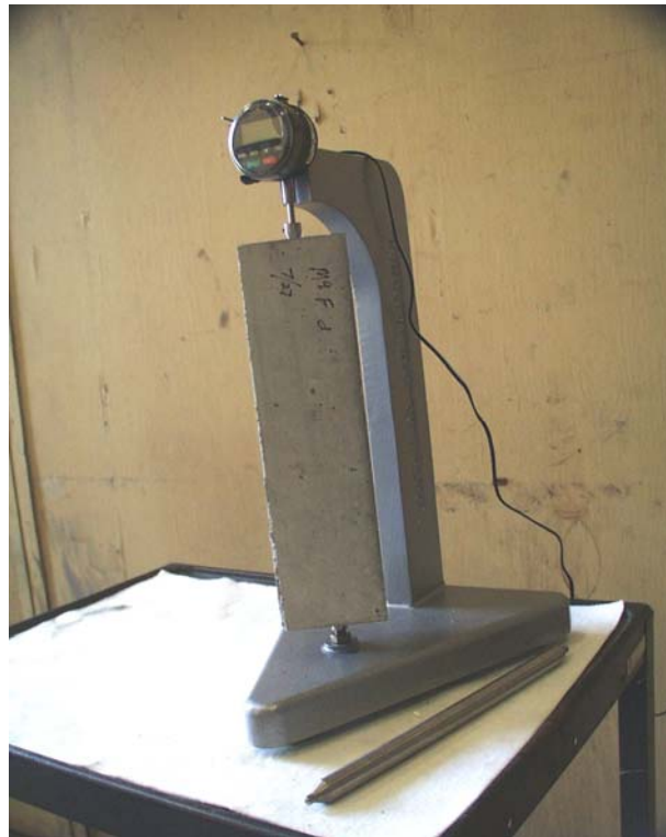
Figure 3-2 Length reading taken with length comparator
