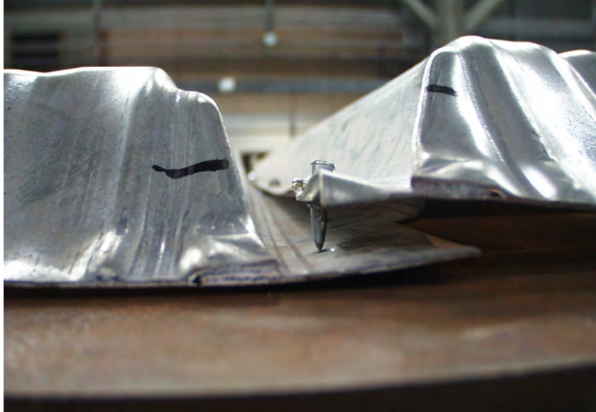
Figure 5.24 Pullout of an End Fastener at a Lap Seam in Test M16-T3
