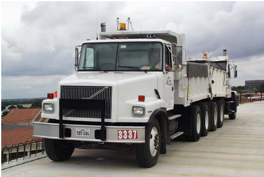
Figure 6.20 Truck Positioning During K Live Load Test
