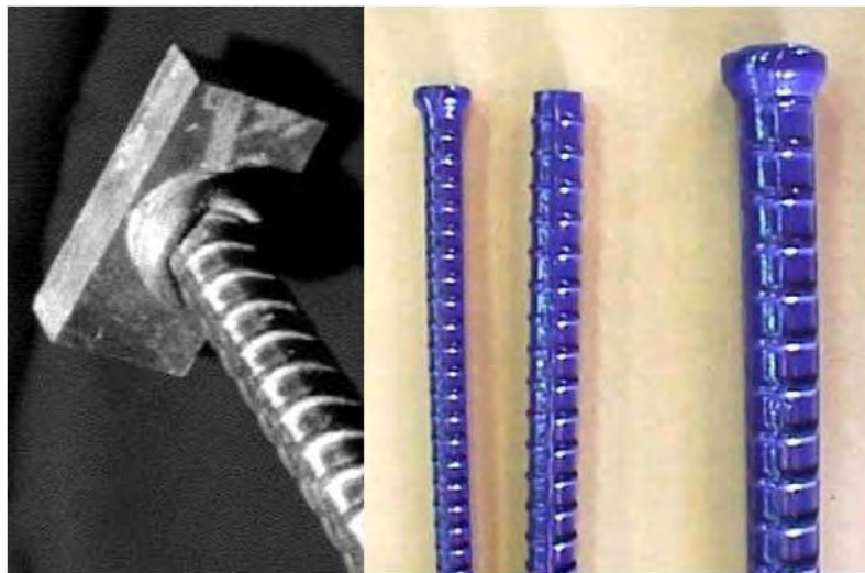
Figure 2.16 T-headed bar and Upset-headed bars [2.11,2.12]
