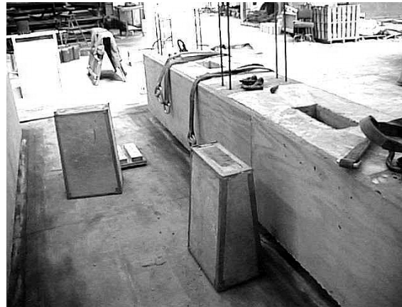
Figure 3.15 Specimen after Removal of Grout Pocket Inserts
