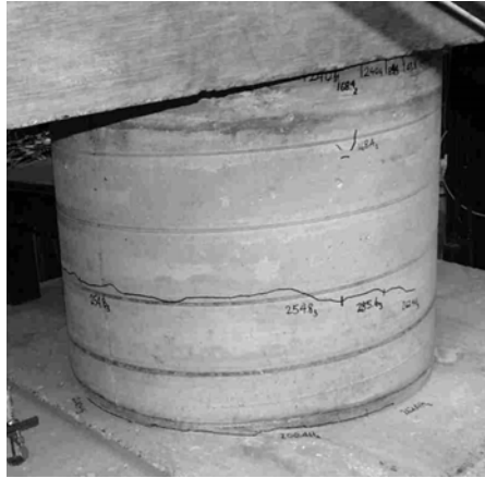
a. Crack on Tension Side
