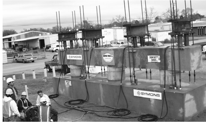
b. Column Bent Test Setup
