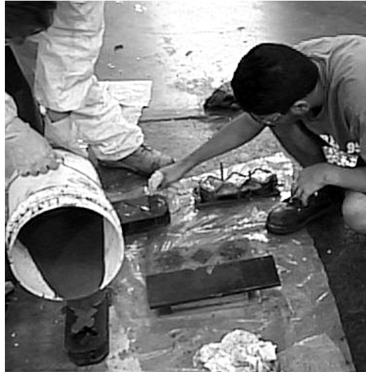
Figure 3.27 Preparation of Grout Cubes
