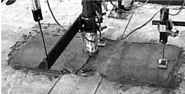
Figure 3.40 Splitting Crack in Grout Pocket (SL03)
