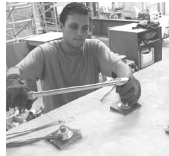
c. Tightening of Bolts
