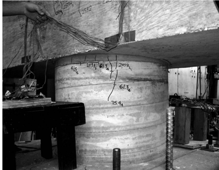
b. Cracks on Compression Side
