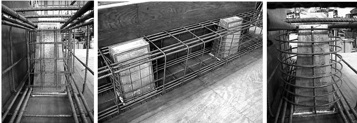
Figure 3.11 Confinement used for Single-Line Grout Pockets
