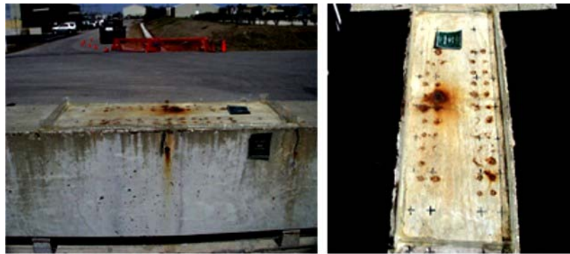
Lateral (South) View Top View (from East Side) Figure 5.36 Specimen 4.2 – Condition Prior to Autopsy 6,7
