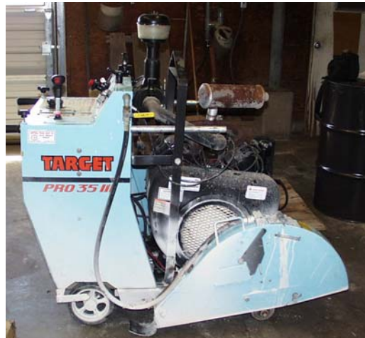
Figure 5.3 Concrete Saw used in Autopsy 6
