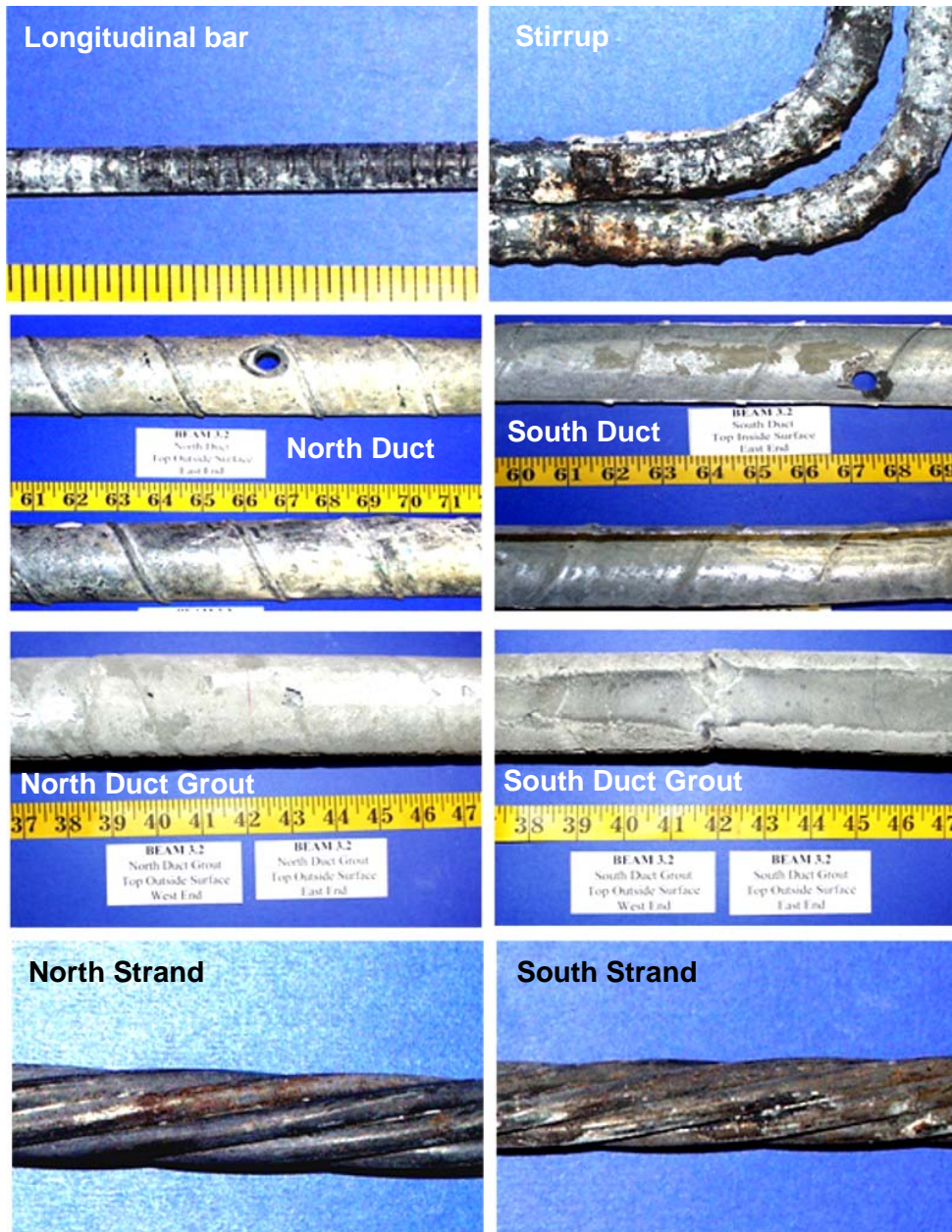
Figure 5.30 Specimen 3.2 – Reinforcing Elements 6,7
