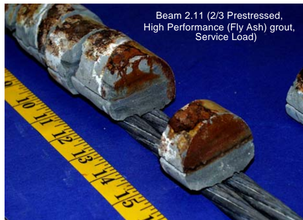
Figure 6.16 Effect of Grout Cracking 7
