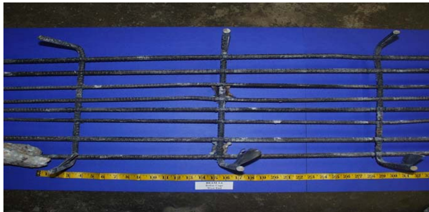
Figure 5.6 Mild Steel Reinforcement Cage
