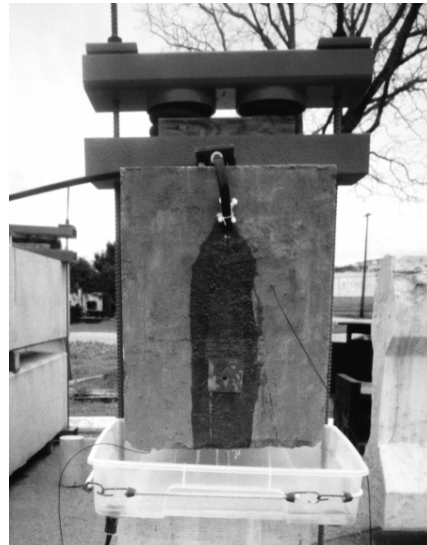
Figure 2.18 Beam End Dripper System 3
