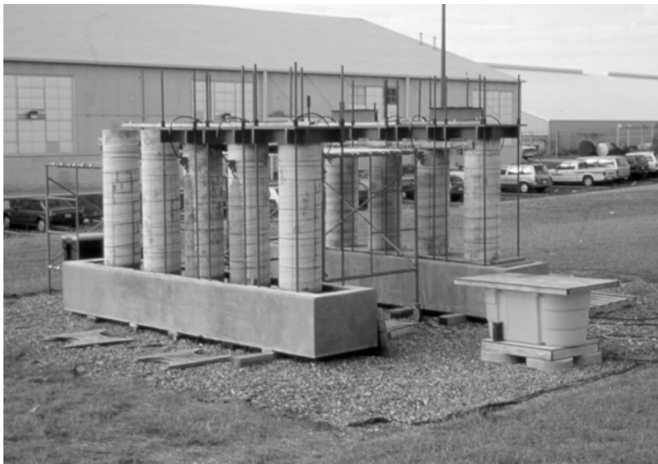
Figure 3.10 - Long-Term Column Corrosion Test Setup
