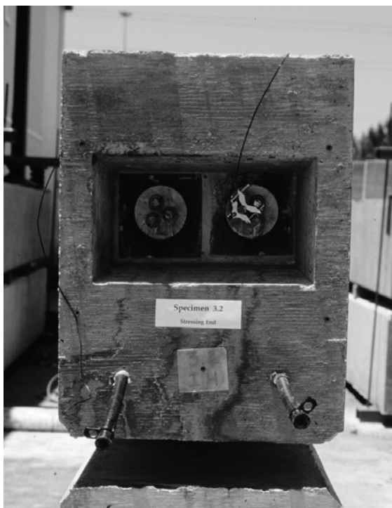
Figure 2.40 - Grouting Tubes for 100% U PS and 100% S PS Sections
