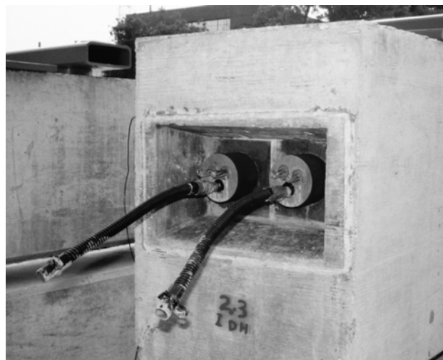
Figure 2.39 - Grouting Tubes for 2/3 PS Specimens
