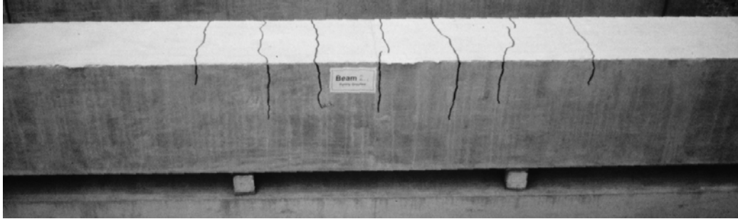
Figure A.43 - Crack Pattern for Specimen 2.9
