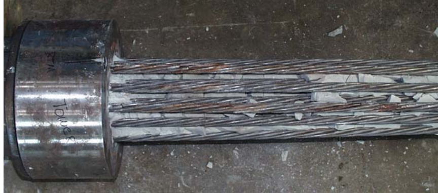
Figure D.149 Corrosion on Surface of Strand near Tower End – Specimen 12
