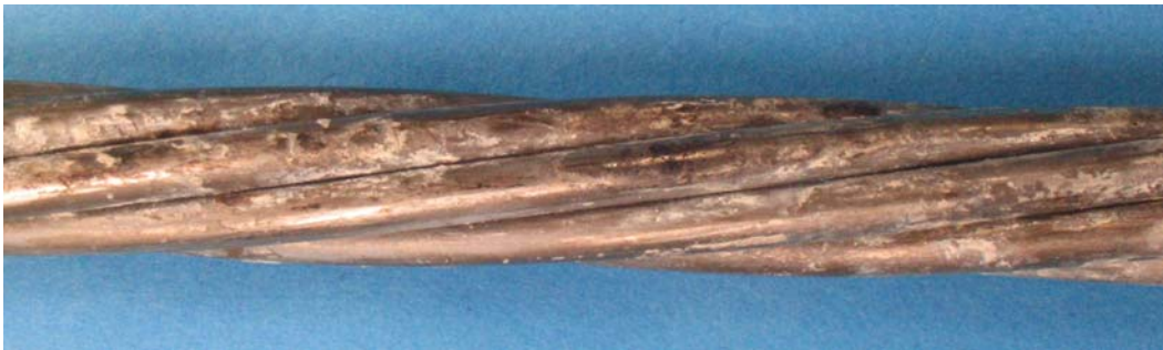
Figure D.78 Corrosion on Surface of Strand 17 at Midspan – Specimen 7
