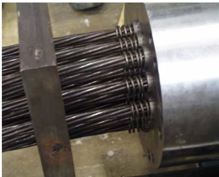
Figure B.26 Spring Plate Used during Stressing
