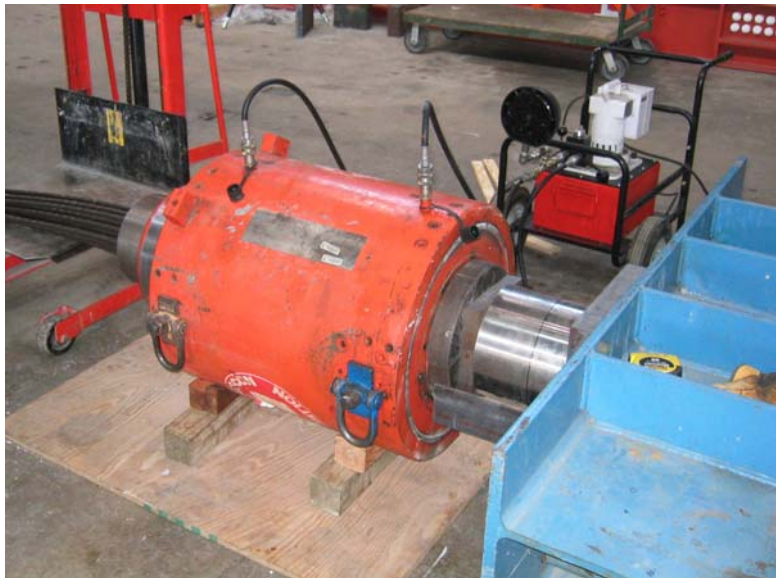
Figure B.25 Hydraulic Ram Used to Stress the Cable-Stay Specimen
