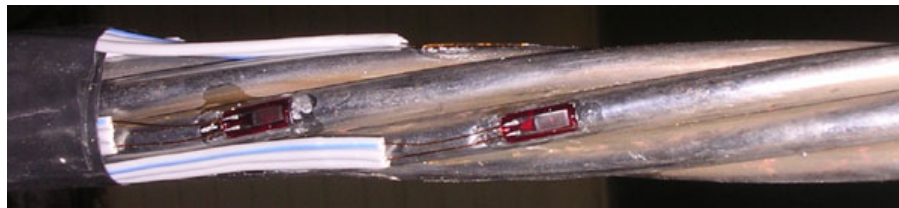
Figure A.11 Strain Gages Positioned along Local Axes of Wires
