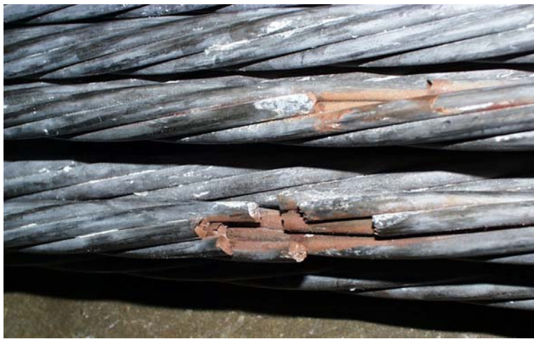
Figure D.124 Corroded Fretting Product near Midspan – Specimen 10
