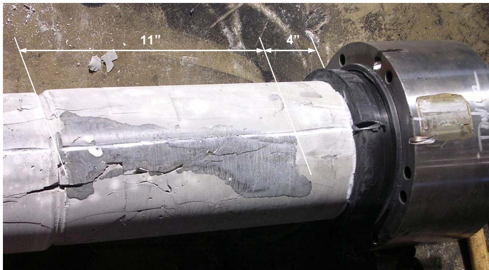
Figure D.105 Intentional Grout Lens at Tower End – Specimen 9
