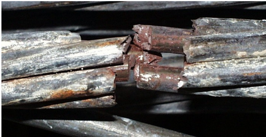
Figure D.60 Corroded Fretting Product on Strand 19 – Specimen 6
