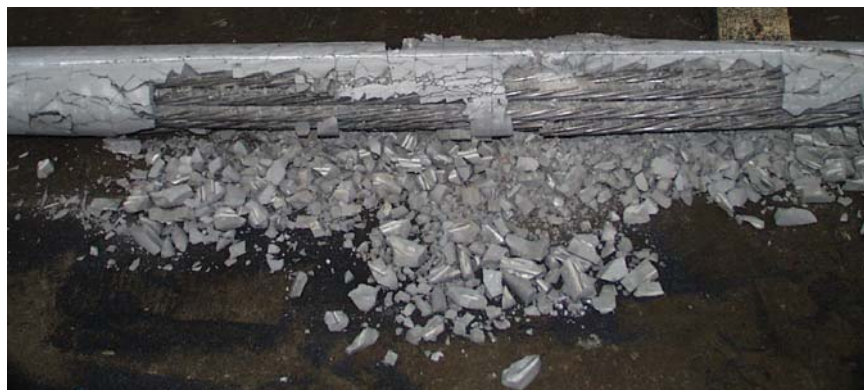
Figure D.146 Condition of Grout near Midspan – Specimen 12
