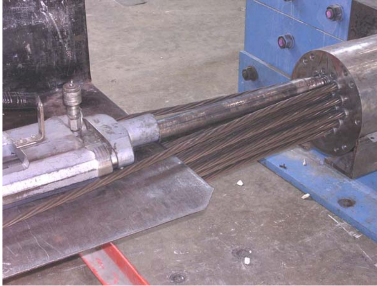
Figure B.24 Application of Initial Prestress to Individual Strands
