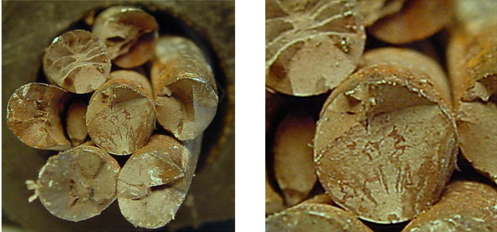
Figure D.24 Fracture Surfaces for Strand 1 near Tower Anchor Head – Specimen 2
