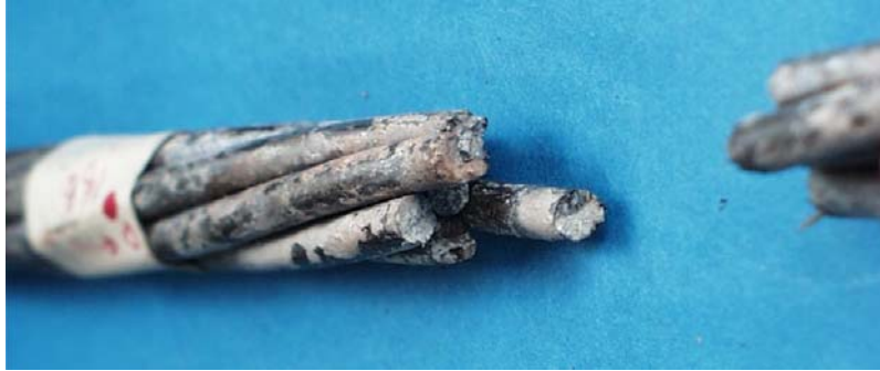
Figure D.77 White Substance on Surface of Strand 17 at Midspan – Specimen 7
