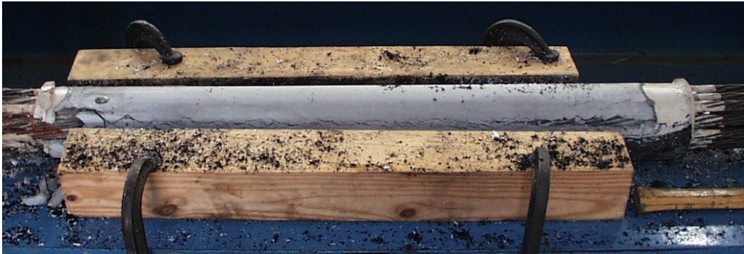
Figure D.50 Condition of Grout in Center Section of Specimen 5
