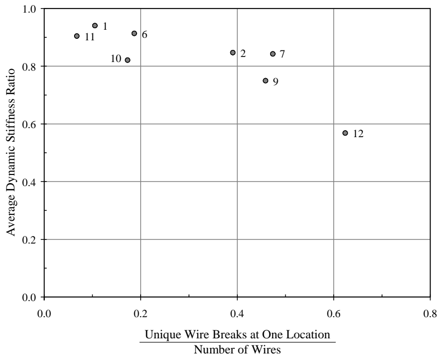
Figure 3.26 Sensitivity of Dynamic Stiffness Ratio to Number of Wire Breaks
