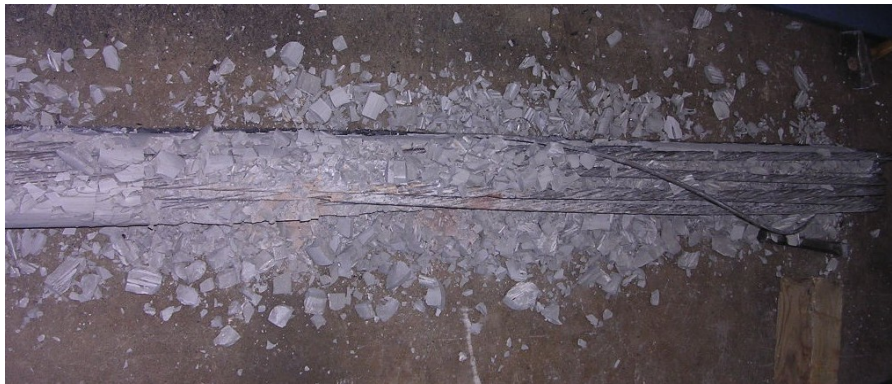
Figure D.107 Condition of Grout under Load Point – Specimen 9
