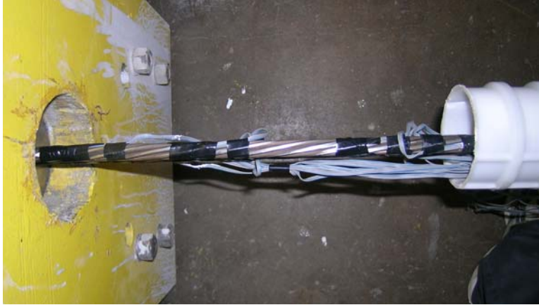
Figure C.12 Strain Gages Attached to Strands at North End of Specimen 1
