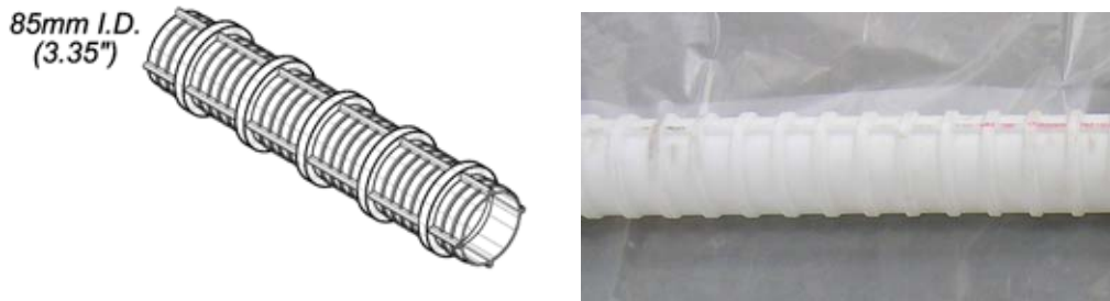
Figure C.6 Post-Tensioning Duct used to Construct Small-Diameter Specimens
