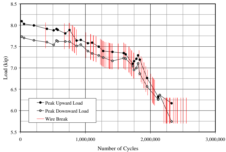
Figure 3.15 Variation of Applied Loads during Fatigue Test of Representative Cable-Stay Specimen
