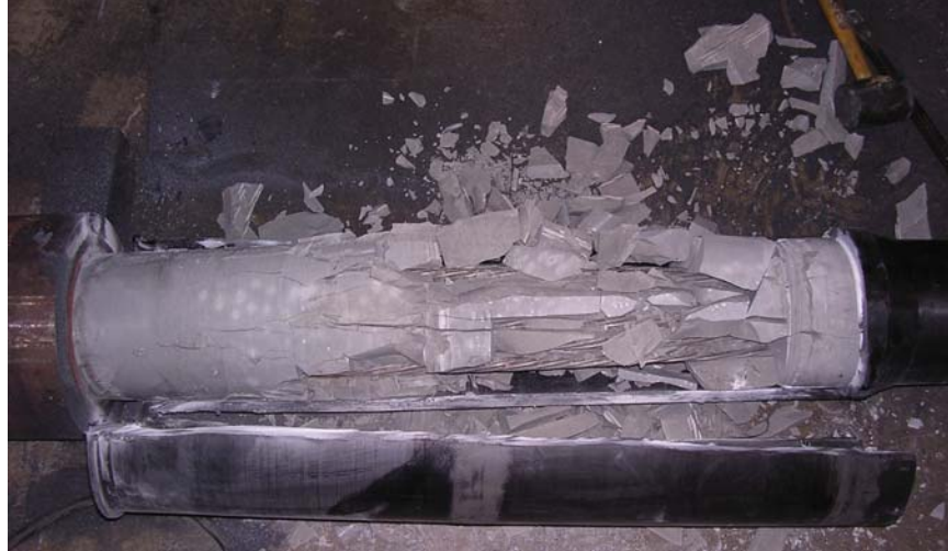
Figure D.147 Condition of Grout near Deck End – Specimen 12
