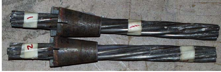
Figure D.152 Corrosion of Wedges at Tower End – Specimen 12
