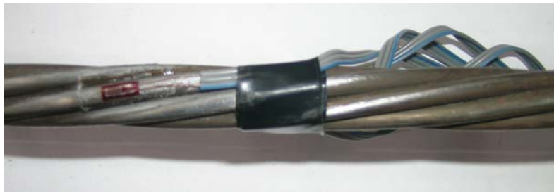
Figure C.13 Strain Gage Oriented along Local Axes of Wire
