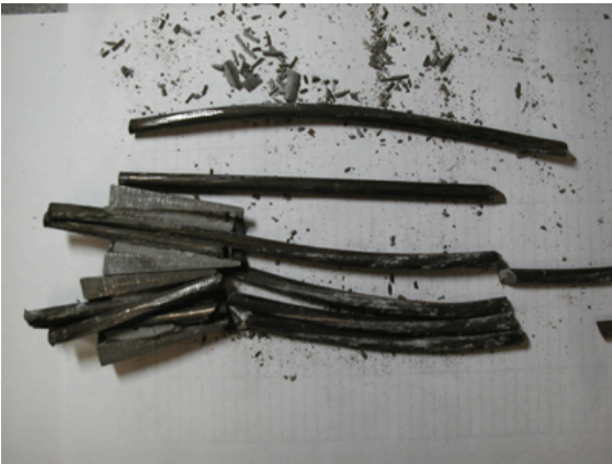
(c) Wire Breaks in Bottom Strand inside Anchor Head
