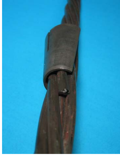
Figure D.101 Wire Break in Strand 11 at Deck End of Specimen 8
