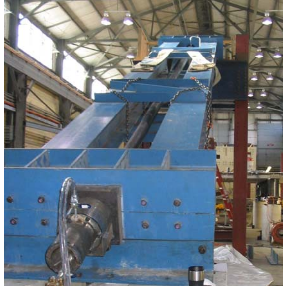
Figure B.27 Grouted Specimen in the Inclined Position for Grouting
