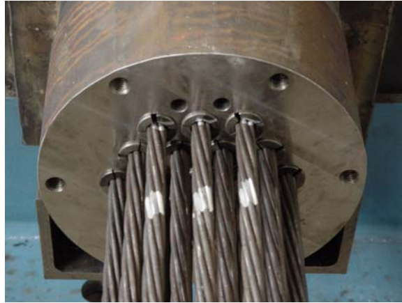
Figure B.22 Installed Wedges
