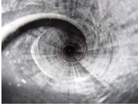
Figure B.19 Helical Spacer Wire inside PE Pipe along Free Length of Specimen
