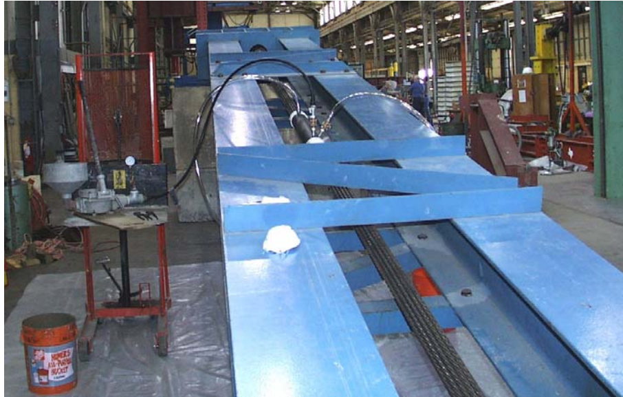
Figure B.29 UngROUTed Specimen in the Inclined Position for Grouting
