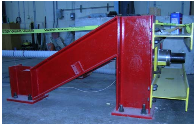
Figure C.2 Reaction Frame and Cross Beams
