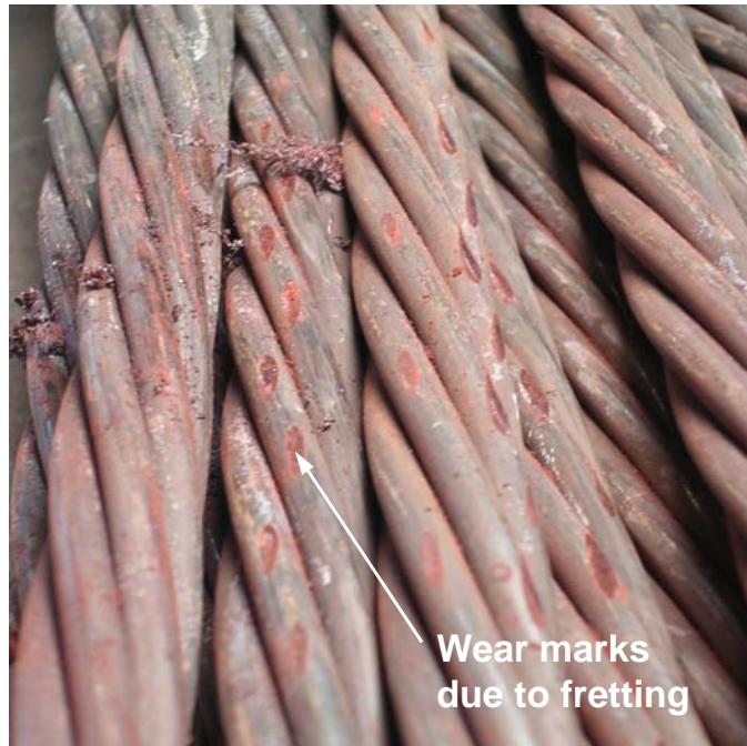
Figure D.92 Reduction of Cross-Sectional Area of Strands Due to Fretting – Specimen 8
